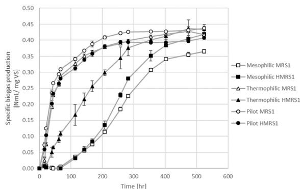
**Fig. 3** Specific biogas production of hydrolysed (HMRS1, filled markers) and non-hydrolysed (MRS1, empty markers) mixed raw sludge in anaerobic digestion assays operated under i) mesophilic conditions with mesophilic inocula (squares), ii) thermophilic conditions with mesophilic inoculum from a full-scale (triangles), and iii) thermophilic conditions and thermophilic inoculum from the pilot (circles).
