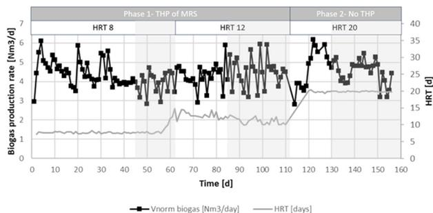
**Fig. 4** Comparison of daily biogas production rates between THP-TAD (phase 1) and conventional TAD (phase 2). The secondary axis depicts the real HRT, with shaded areas indicating stabilised operation periods.
