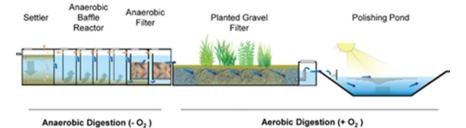
Fig. 14 Pretreatment of wastewater prior to UV disinfection.
