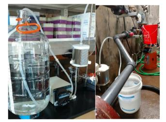
Fig. 35 UV LED reactor disinfection performance was assessed under varying conditions at bench scale (left) to develop a predictive model that was used to assess performance during challenge testing after pilot installation (right).
