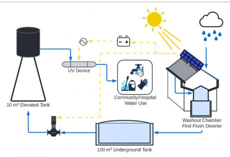
Fig. 31 UV rainwater harvesting (UV RWH) system.
