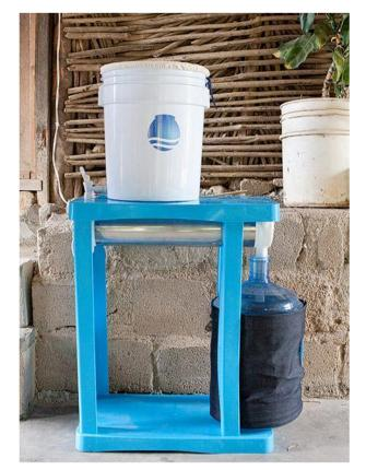
Fig. 19 Mesita Azul household water treatment system with an openchannel UV reactor (silver cylinder) fed by gravity.
