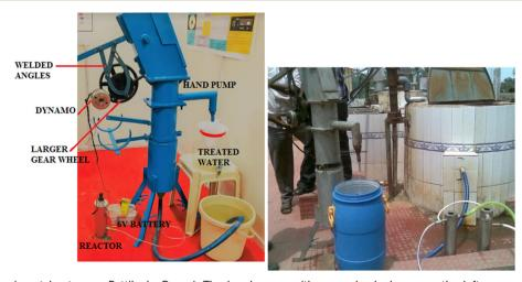
Fig. 11 Fitting of experimental setup on Pattikadu Oorani. The hand pump with gear wheel, shown on the left, was modified to drive a gear system linked to a dynamo, converting mechanical energy into electricity and charging a 6 V DC battery. The UV LED reactor is the silver cylinder in the bottom right of the right photo.
