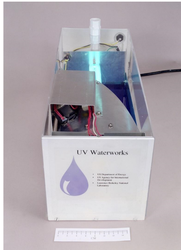
Fig. 13 UV waterworks, built with a glass cover for exhibits and displays to explain how the technology works.
