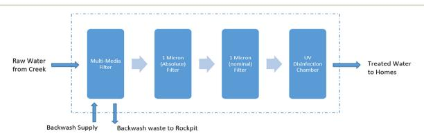
Fig. 2 The Lytton POE systems process flow diagram.
