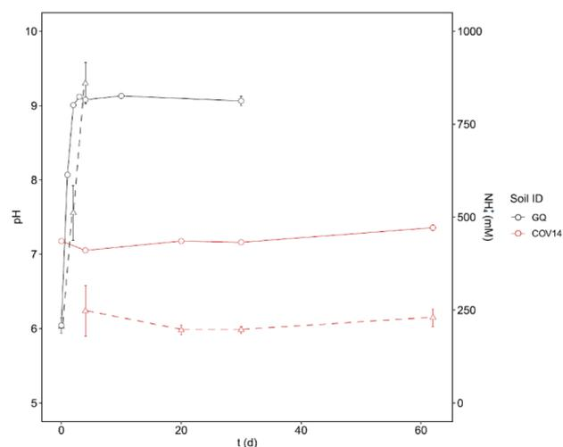
**Fig. 2** Evolution of soil pH (left y-axis, circle) and NH<sub>4</sub><sup>+</sup> (right y-axis, triangle) over time following application of treatment to induce urea hydrolysis on an uncontaminated quarry sand (GQ) and a polluted soil from a gas plant (COV14). Markers and error bars indicate the average and standard deviation of three replicate samples.
