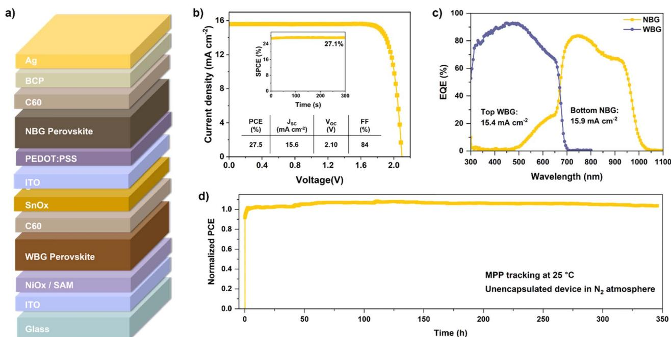
Fig. 5 (a) Schematic illustration of the architecture for all-perovskite tandem solar cells (APTSCs). (b)  $J$ - $V$  curve and the SPCE of the champion APTSC under continuous AM 1.5G illumination. (c) The external quantum efficiency (EQE) curves of the APTSCs. (d) MPP tracking of a non-encapsulated APTSC under AM 1.5G illumination in N<sub>2</sub> atmosphere at 25 °C.
