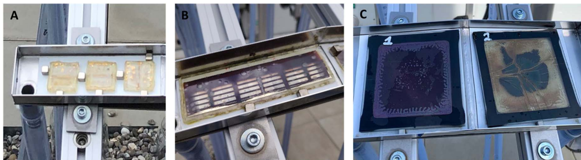
Fig. 2 Mini-glass samples (A), plastic samples (B) and large-area samples (C) at the end of outdoor experiments.
