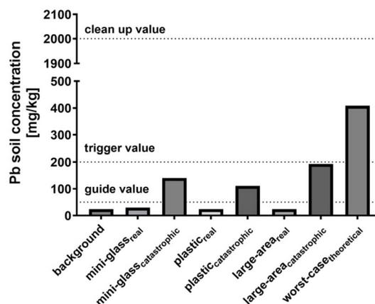
Fig. 3 Resulting Pb soil concentrations for the leaching scenarios considered (for details refer to text). Legislative values in terms of soil protection in Switzerland (*i.e.* guide value, trigger value and clean-up value) are indicated by dotted lines. Note that the y-axis is broken, and even the theoretical worst-case would result in Pb soil concentrations approximately four times lower than the clean-up value specified by Swiss regulations.
