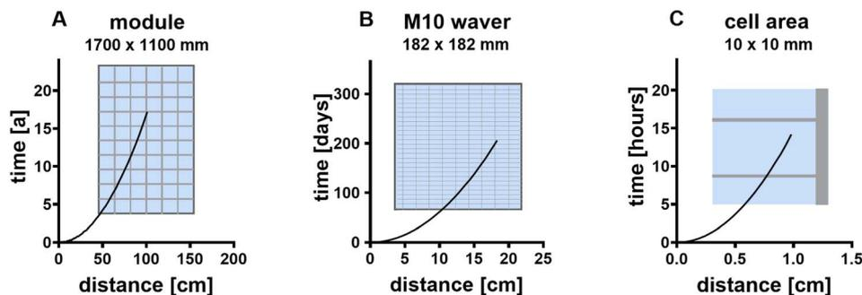
Fig. 4 Diffusion times for the Pb cation in pure H<sub>2</sub>O in relation to typical dimensions in PV such as a full module (A), a single wafer (B) and a cell area of 1 cm<sup>2</sup> (C). Note that fingers and busbars are not drawn to dimension.
