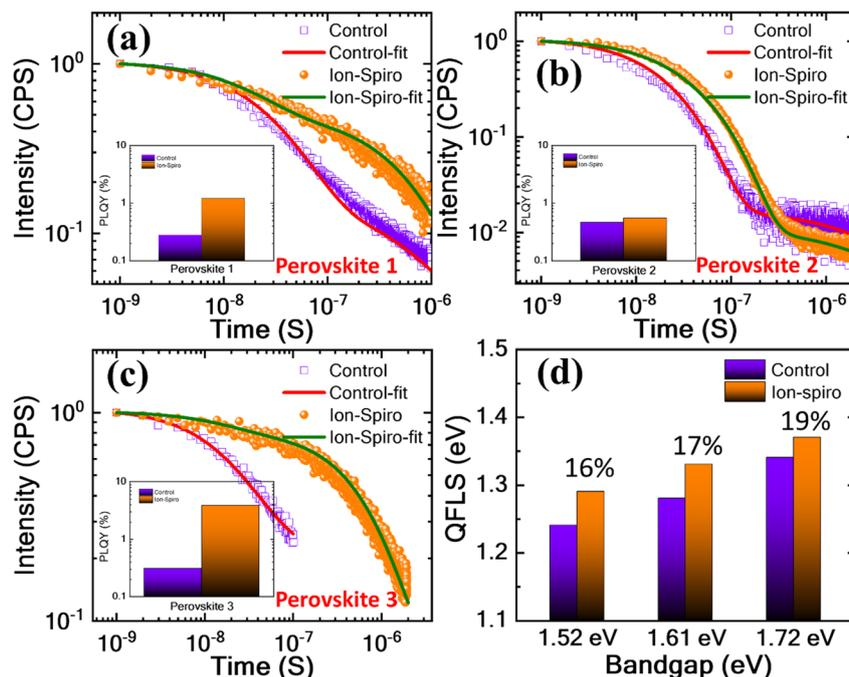
Fig. 3 Optical analysis of the bandgap varying transparent semi-processed PSCs (glass/FTO/SnO<sub>2</sub>/perovskite/control or Ion-Spiro HTL) with control and ion-modulated spiro-MeOTAD HTL. Fitted TCSPC carrier lifetime decay with PLQY (inset) of (a) perovskite 1, (b) perovskite 2, and (c) perovskite 3. (d) Estimated QFLS of variable bandgap transparent PSCs with the control and ion-modulated spiro-MeOTAD HTL.
