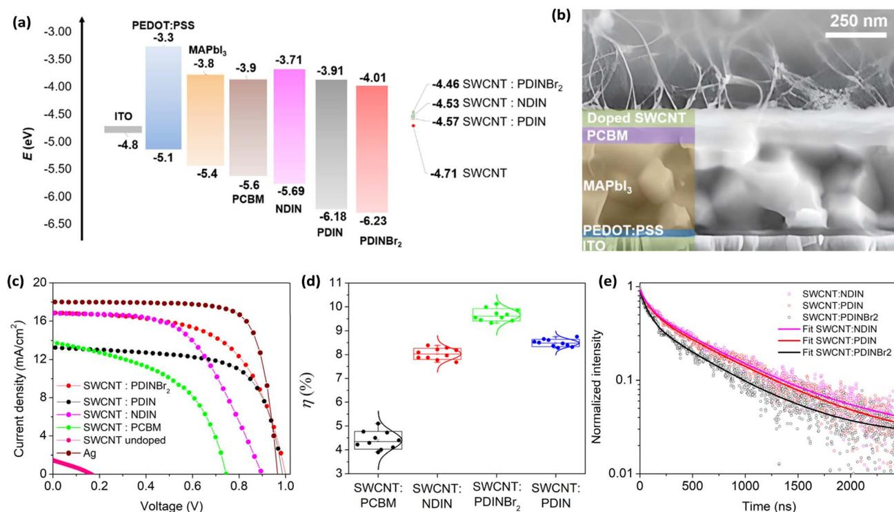
Fig. 4 (a) Energy level diagram of the inverted perovskite solar cell, (b) their cross-sectional SEM image, (c) comparison of  $J$ - $V$  characteristics of inverted perovskite solar cells incorporating different cathodes, (d) statistical distributions of power conversion efficiency, and (e) microwave photoconductivity decay ( $\mu$ -PCD) profiles of ITO/MAPbI<sub>3</sub>/PCBM/n-doped SWCNT bilayers.
