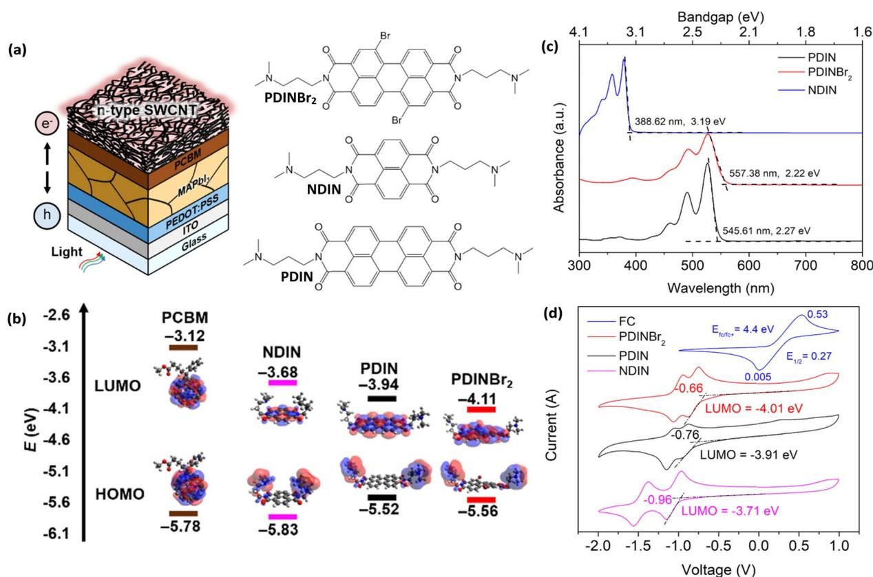
Fig. 1 (a) Device architecture of an inverted PSC utilizing a PDIN/PDINBr<sub>2</sub>/NDIN doped SWCNT cathode, (b) DFT calculated HOMO–LUMO energy of PCBM, NDIN, PDIN, and PDINBr<sub>2</sub>, (c) UV-vis spectra of PDIN, PDINBr<sub>2</sub>, and NDIN measured in TFE and (d) their cyclic voltammetry plot in 0.1 M NBu<sub>4</sub>PF<sub>6</sub>/ODCB, with Fc/Fc<sup>+</sup> as the internal reference.
