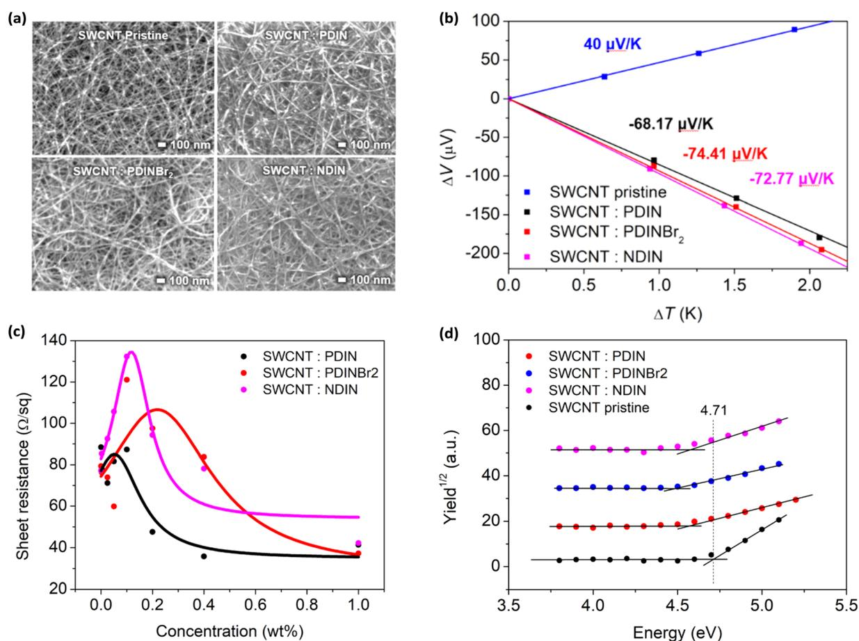
Fig. 3 (a) SEM images of pristine and doped SWCNT film, (b) plots of thermoelectric voltage ( $\Delta V$ ) versus the applied temperature difference ( $\Delta T$ ) of pristine and doped SWCNT films, (c) correlation between sheet resistance and doping concentration in SWCNT films, and (d) PYSA spectra of pristine and doped SWCNT films.
