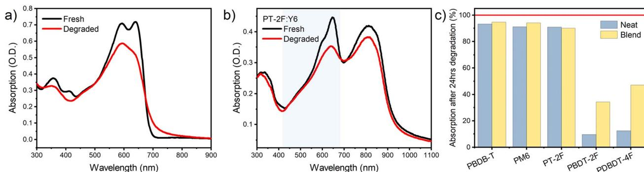
**Fig. 2** Film absorption spectra of neat **PT-2F** (a) and **PT-2F** blends with Y6 (b) before and after 24 hours of 1 sun illumination in ambient air; (c) the integrated absorption of all neat polymer and Y6-blend films after degradation relative to the fresh absorption; for blend films the blue-shaded area in (b) shows the wavelength range used for integration of the specific polymer absorption.
