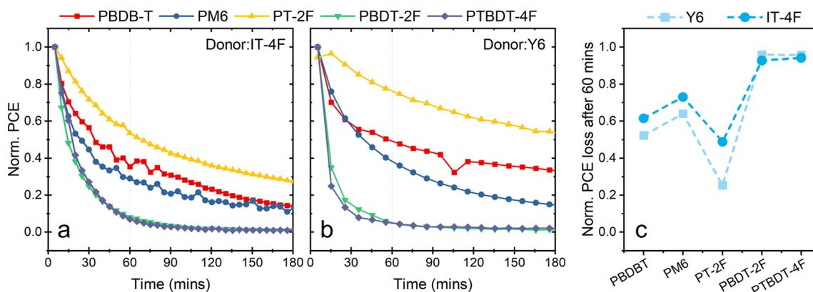
Fig. 3 Device stability of the PBDB-T class of polymers. (a & b) Average, normalised power conversion efficiencies (PCE) of ITO/ZnO/Donor: Acceptor/MoO<sub>3</sub>/Ag devices as a function of illumination time in air; (c) normalised PCE loss of these devices after 60 minutes ageing.
