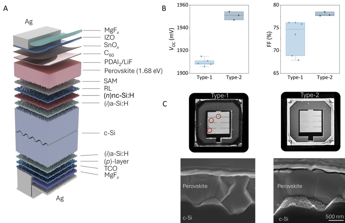
**Fig. 1** (A) The schematic of the monolithic perovskite–silicon tandem device, (B) the  $V_{OC}$  and FF of the fabricated tandem devices featuring different bottom cells, with Type-1 and Type-2 based on 15-nm-thick and 25-nm-thick ( $n$ )nc-Si:H layers, respectively, and (C) the PL images and cross-sectional SEM micrographs of respective devices. Note that Type-1 features 10-nm-thick ITO and Type-2 has 5-nm-thick IZO as the interconnecting recombination layer (RL) and rear TCO layer.
