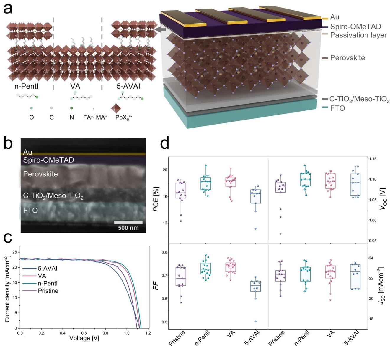
Fig. 4 Device architecture and performance. (a) Schematic of the device structure. (b) Cross-section SEM image of the device. (c)  $J$ - $V$  curves (reverse scans) of the champion PSCs without and with passivation layers. (d) Statistical distributions of photovoltaic parameters of PSCs based on the pristine perovskite layer and perovskite layer passivated with *n*-PentI, VA, and 5-AVAI.
