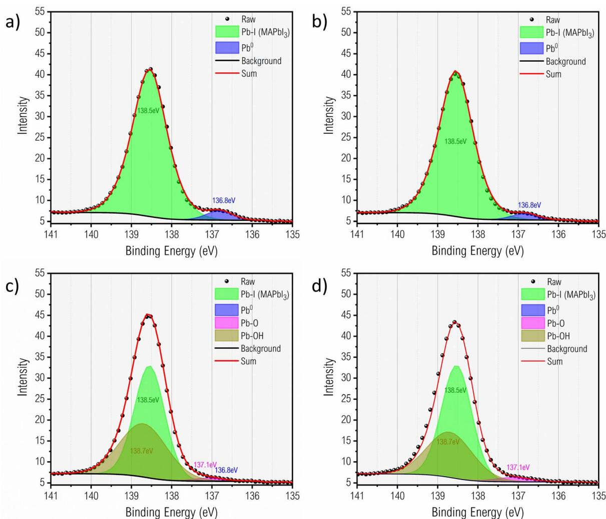
Fig. 3 XPS Pb  $4f_{7/2}$  region of (a) Primary-MAPbI<sub>3</sub>, (b) 2nd-MAPbI<sub>3</sub>/dry, (c) 2nd-MAPbI<sub>3</sub>/wet and (d) 2nd-MAPbI<sub>3</sub>/heat films.
