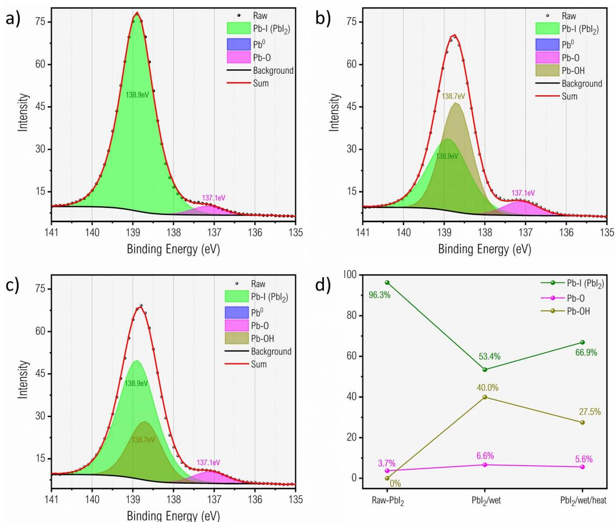
Fig. 6 (a)–(c) XPS Pb 4f<sub>7/2</sub> regions and (d) binding ratios of Raw-PbI<sub>2</sub>, PbI<sub>2</sub>/wet, PbI<sub>2</sub>/wet/heat films.
