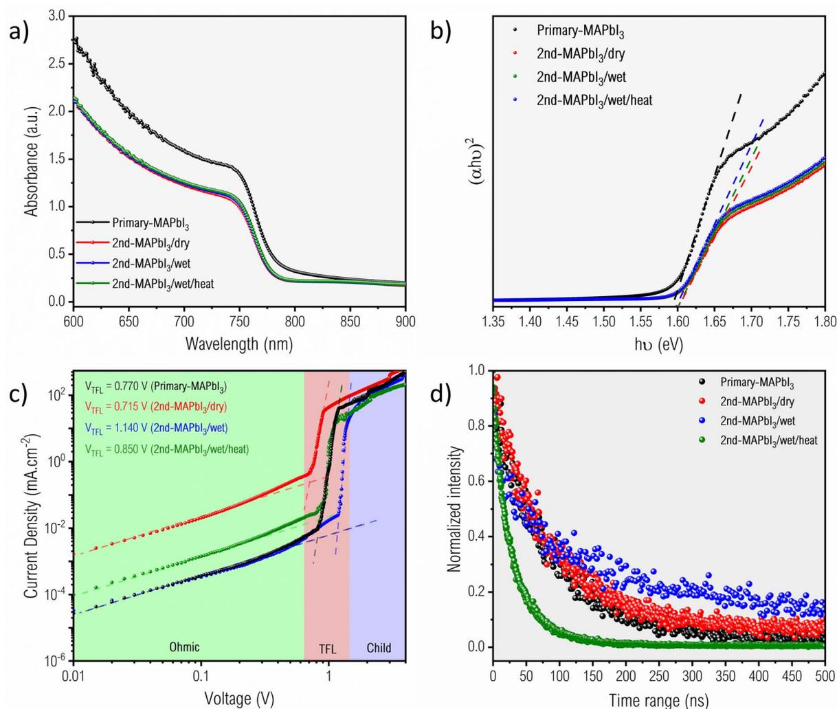
Fig. 8 (a) UV-vis absorption spectra, (b) Tauc-plot, (c) the SCLC curves and (d) the TRPL spectra of the glass/ $\text{Al}_2\text{O}_3$ /PVSK film of Primary-MAPbI<sub>3</sub>, 2nd-MAPbI<sub>3</sub>/dry, 2nd-MAPbI<sub>3</sub>/wet and 2nd-MAPbI<sub>3</sub>/wet/heat films.
