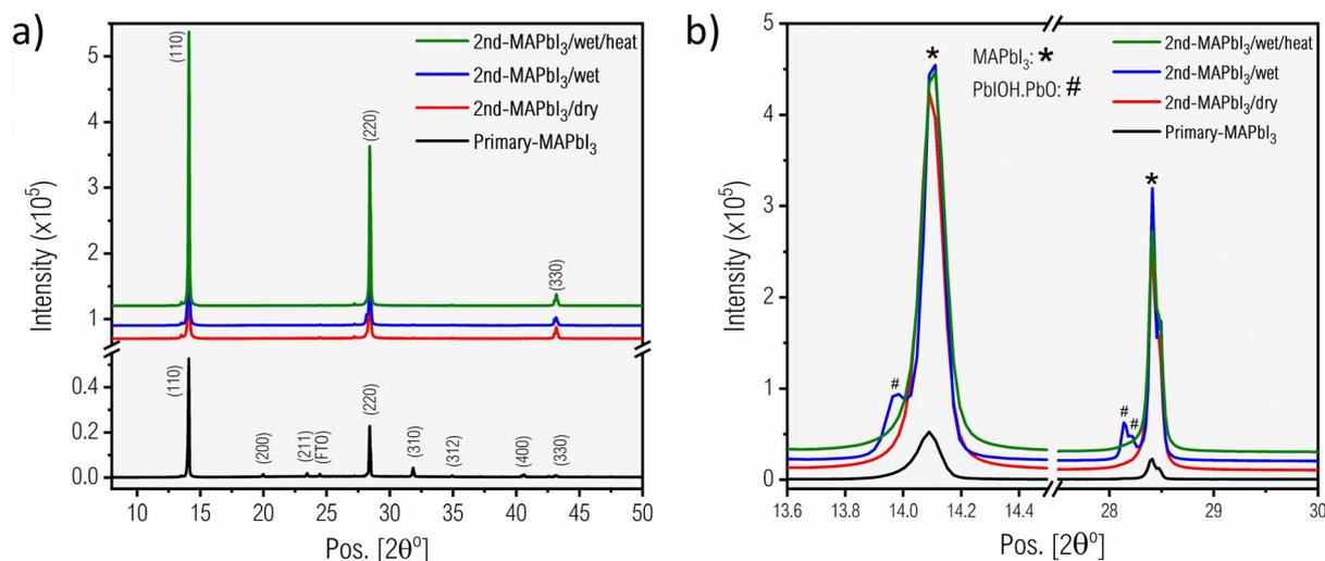
Fig. 2 (a) XRD pattern and (b) zoom-in peak at  $14.0^\circ$  and  $28.5^\circ$  of Primary-MAPbI<sub>3</sub>, 2nd-MAPbI<sub>3</sub>/dry, 2nd-MAPbI<sub>3</sub>/wet and 2nd-MAPbI<sub>3</sub>/heat films.
