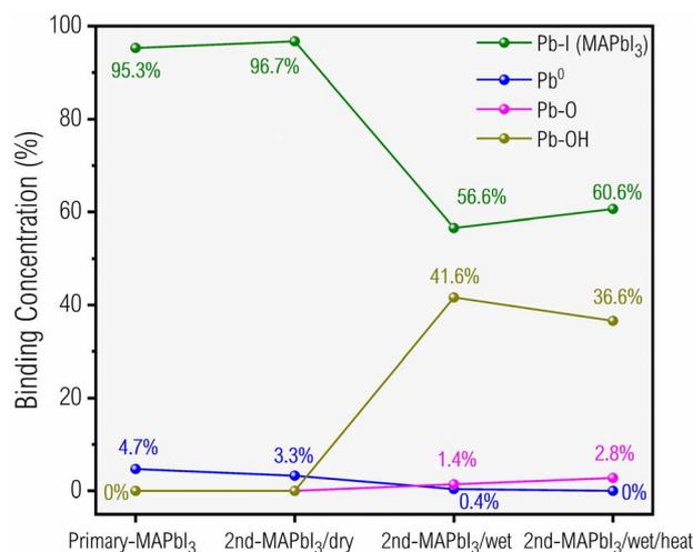
Fig. 4 Pb binding ratios of four types of MAPbI<sub>3</sub> films obtained from the deconvoluted Pb  $4f_{7/2}$  spectra.
