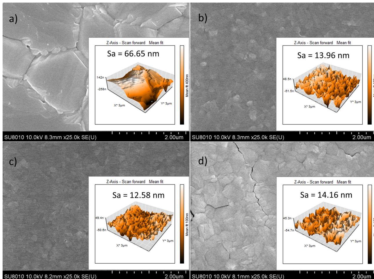
Fig. 7 SEM topographic view and AFM of PVSK films: (a) Primary-MAPbI<sub>3</sub>, (b) 2nd-MAPbI<sub>3</sub>/dry, (c) 2nd-MAPbI<sub>3</sub>/wet and (d) 2nd-MAPbI<sub>3</sub>/wet/heat films.
