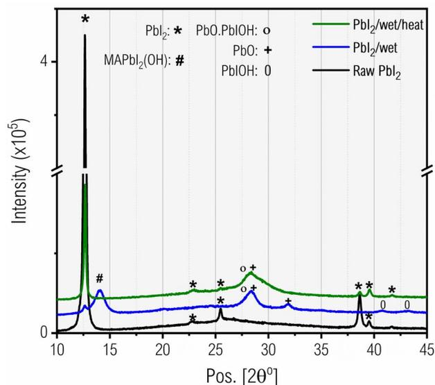
Fig. 5 XRD patterns of Raw-PbI<sub>2</sub>, PbI<sub>2</sub>/wet and PbI<sub>2</sub>/wet/heat films.
