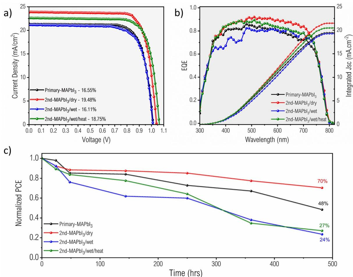
Fig. 9 (a) The best performance  $J$ – $V$  curves of perovskite MAPbI<sub>3</sub> devices with Primary-MAPbI<sub>3</sub> and 2nd-MAPbI<sub>3</sub> (backward scan); (b) EQE and integrated  $J_{sc}$  of perovskite MAPbI<sub>3</sub> devices and (c) stability of devices made using Primary-MAPbI<sub>3</sub> and 2nd-MAPbI<sub>3</sub> films.
