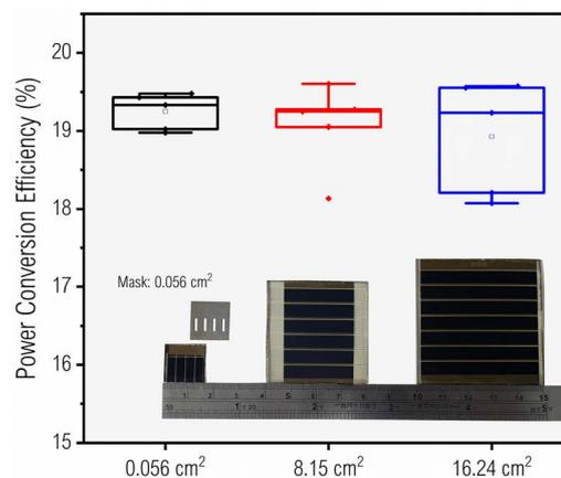
Fig. 10 Performance of small devices and module devices.
