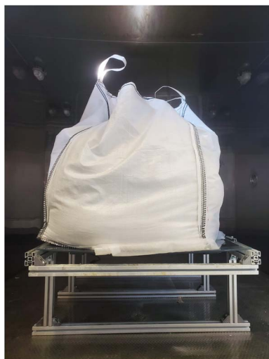
Fig. 7 Setup for the mechanical load testing in the climate chamber. The weight was evenly distributed with sand-filled bags.
