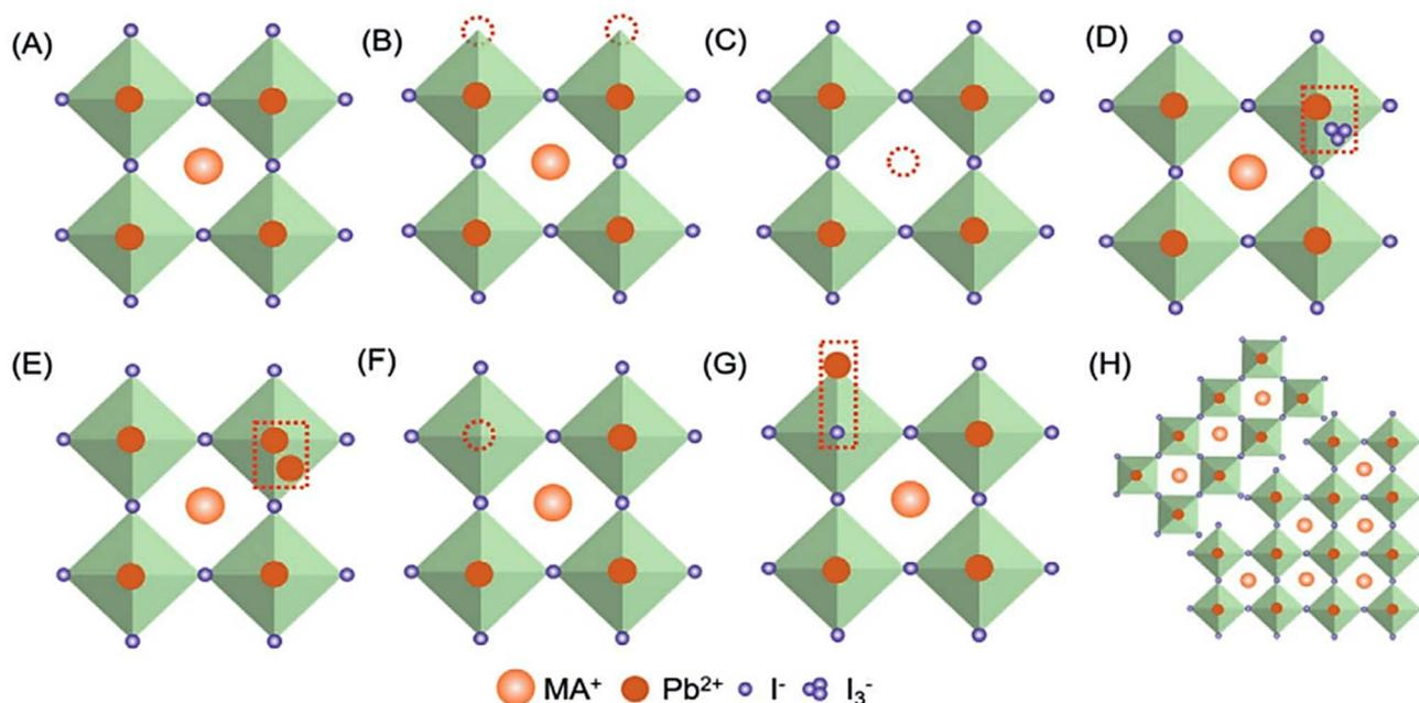
Fig. 9 Representative defect types in perovskite solar cells. (A) Ideal crystal structure, (B) iodide vacancy, (C) methylammonium ( $\text{MA}^+$ ) vacancy, (D) triiodide ( $\text{I}_3^-$ ) interstitial, (E) lead ( $\text{Pb}^{2+}$ ) interstitial, (F) lead vacancy, (G) Pb–I anti-site defect, and (H) grain boundary. Reproduced with permission from ref. 69 Copyright 2021 Wiley-VCH GmbH.
