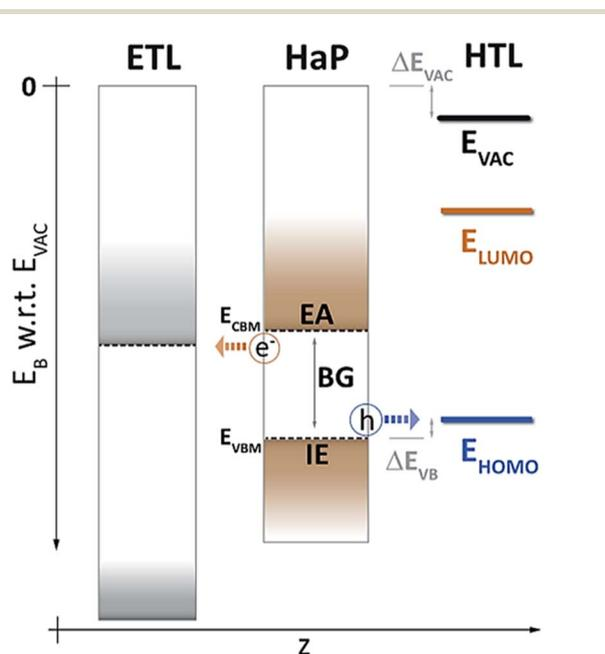
Fig. 11 Fundamental energies like ionization energy (IE) and electron affinity (EA), along with the positions of band edges ( $E_{CBM}$  and  $E_{VBM}$ ) of a perovskite layer with a specific band gap (BG) compared to energy levels of adjacent charge transport layers. Reproduced with permission from ref. 78, Copyright 2014. Royal Society of Chemistry.
