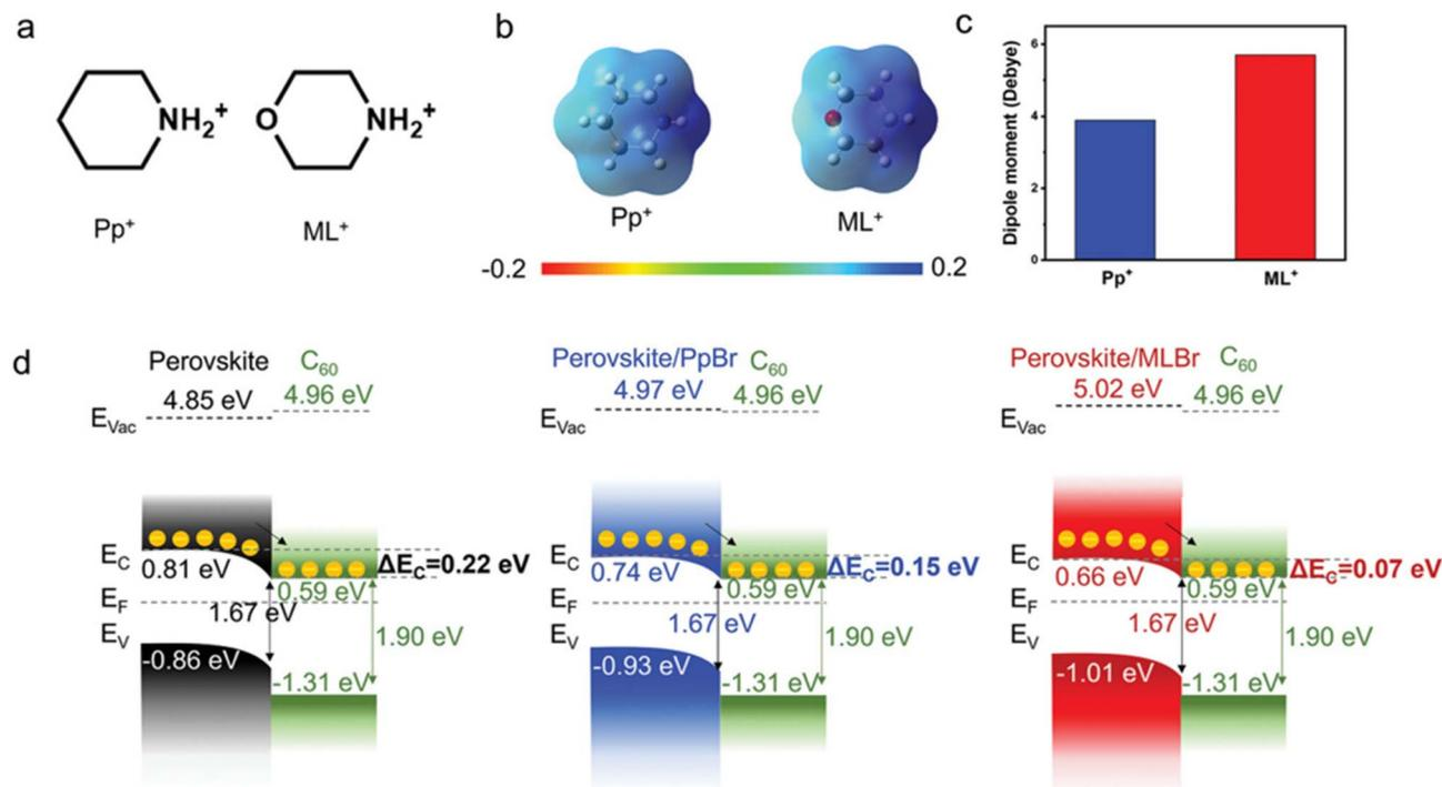
Fig. 40 Dipole engineering at the perovskite/C<sub>60</sub> interface. (a) Molecular structures of Pp<sup>+</sup> and ML<sup>+</sup>. (b) Electrostatic potential (ESP) distributions. (c) Calculated dipole moments. (d) Energy level alignment for perovskite/C<sub>60</sub>, perovskite/PpBr/C<sub>60</sub>, and perovskite/MLBr/C<sub>60</sub> configurations. Reproduced with permission from ref. 205. Copyright 2024 Wiley-VCH GmbH.
