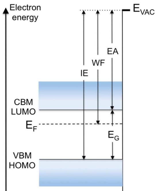
Fig. 10 Semiconductor's energy diagram showing flat bands on the surface. Vacuum level  $E_{VAC}$ , WF, energy gap  $E_G$ , ionization energy IE, band edges (CBM/LUMO and VBM/HOMO), and electron affinity EA are defined. Images reproduced with permission from ref. 73, Copyright 2015. Royal Society of Chemistry.
