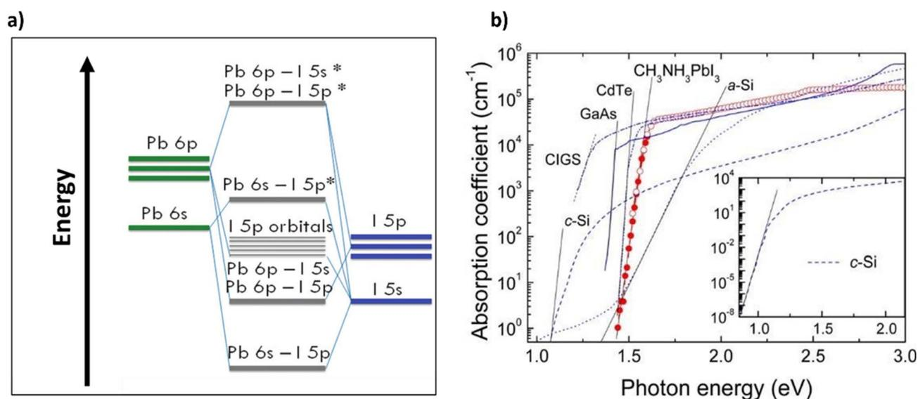
Fig. 4 (a) Schematic depiction of the molecular orbital energy levels of  $\text{MAPbI}_3$  perovskite; reproduced with permission from ref. 23 Copyright 2015, Royal Society of Chemistry; (b) absorption coefficient comparison between  $\text{MAPbI}_3$  and other representative light-harvesting materials. Reproduced with permission from ref. 8 Copyright 2014, American Chemical Society.
