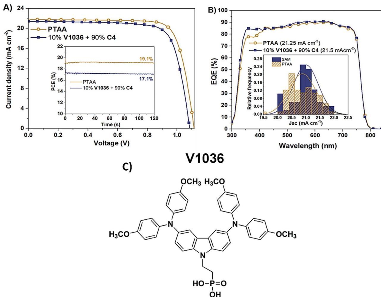
Fig. 16 Photovoltaic performance and spectral response of SAM-modified PSCs. (a)  $J$ - $V$  curves and MPP tracking of PTAA devices with V1036/C4 SAMs; (b) EQE spectra of PTAA and SAM-HTM hybrids; (c) structure of a V1036 molecule. Reproduced with permission from ref. 129, Copyright 2018 WILEY-VCH Verlag GmbH & Co.
