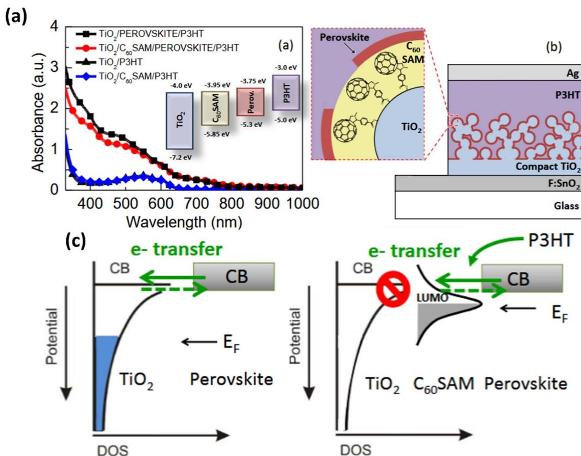
Fig. 15 Impact of  $C_{60}$ -SAM functionalization on perovskite optoelectronics and charge transfer: (a) absorption spectra of P3HT/perovskite films with and without  $C_{60}$ -SAM modification; (b) schematic of the device architecture; (c) energy level diagram illustrating electron transfer pathways, with shaded DOS regions indicating occupied states in  $TiO_2$  and fullerene layers. Reproduced with permission from ref. 127 Copyright 2013, American Chemical Society.
