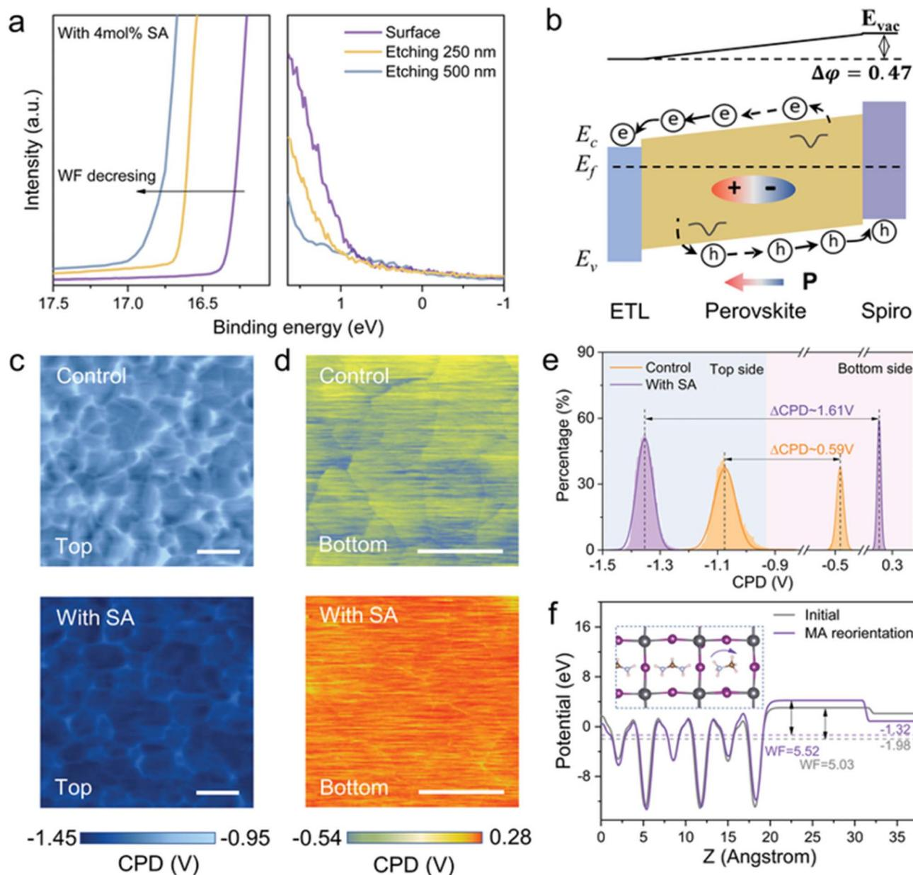
Fig. 39 Electronic properties and charge transport. (a) UPS spectra of SA-regulated perovskite films recorded at different  $\text{Ar}^+$  ion etching depths. (b) Energy-level diagram and carrier transport model. (c and d) KPFM CPD maps of top and bottom film surfaces. (e) Histogram of CPD values. (f) Calculated electrostatic potential and WF with/without  $\text{MA}^+$  reorientation. Reproduced with permission from ref. 204, Copyright 2023 Wiley-VCH GmbH.
