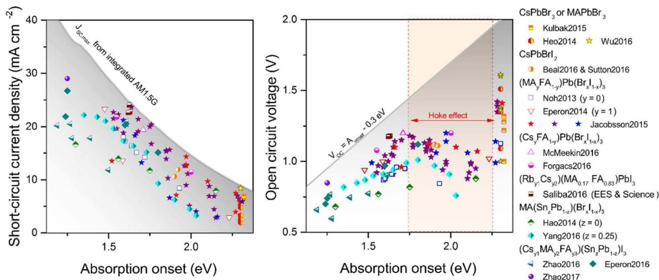
Fig. 6 Experimental  $J_{\text{SC}}$  values as a function of the perovskite absorber bandgap ( $E_g$ ) benchmarked against the theoretical radiative limit (left). Correlation between  $V_{\text{OC}}$  and  $E_g$  (right). Reproduced with permission from ref. 37 Copyright 2017, Royal Society of Chemistry.
