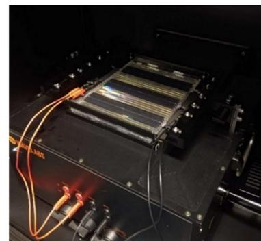
Fig. 12 (a) Spectrally selective APV module concept with DBR embedded layer. (b) Small scale prototype under test in a solar simulator.
