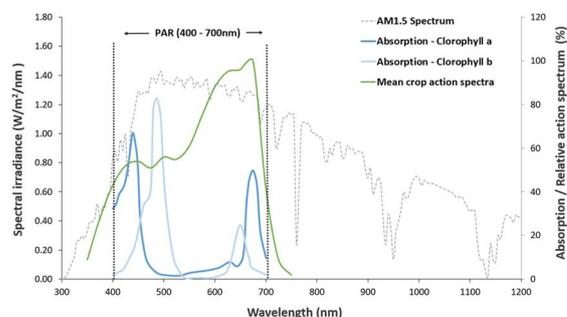
Fig. 2 Chlorophyll absorption and mean crop action spectra compared to AM1.5 spectrum. Crop action spectra data taken from ref. 39.
