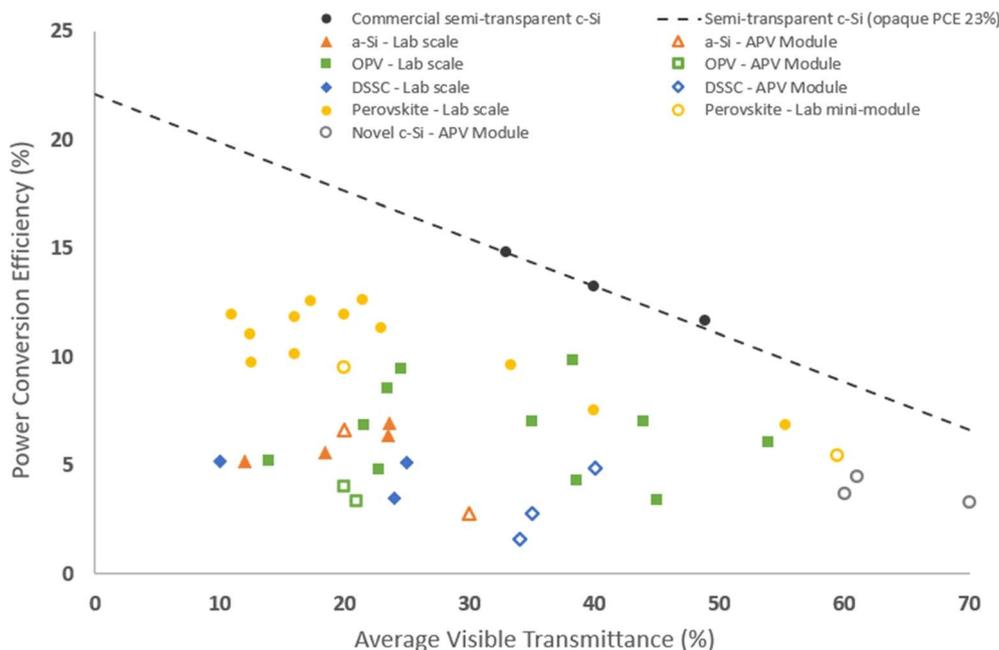
Fig. 9 PCE as a function of AVT for laboratory scale thin film solar cells as reported by Lee *et al.*,<sup>84</sup> Subhani *et al.*<sup>100</sup> and Jafarzadeh *et al.*,<sup>99</sup> solid markers; and for semi-transparent APV technologies demonstrated at the module or mini-module scale reviewed herein, hollow markers. Included for comparison are results for commercially available partially populated c-Si modules.
