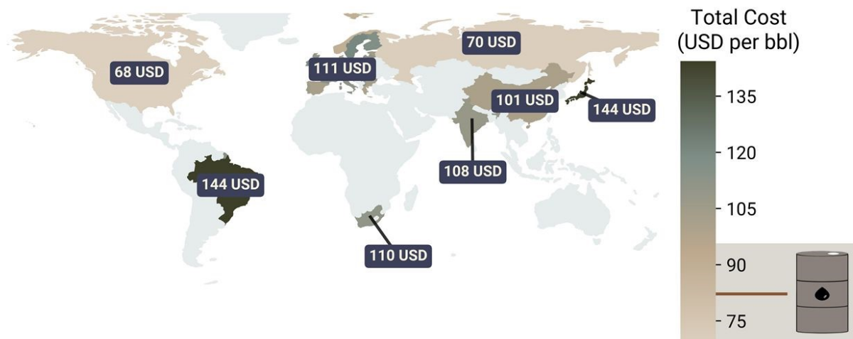
Fig. 4 Regional cost of heating and electricity impacts the biogas-derived syncrude economic potential. Cost per barrel of syncrude from biogas, based on regional feedstock prices. Regional data on natural gas and electricity prices were used, as described in Table S17 of the SI. For the lower range of biogas costs, bio-syncrude would have the potential to outperform crude oil (the range given corresponds to the price variability in 2024).
