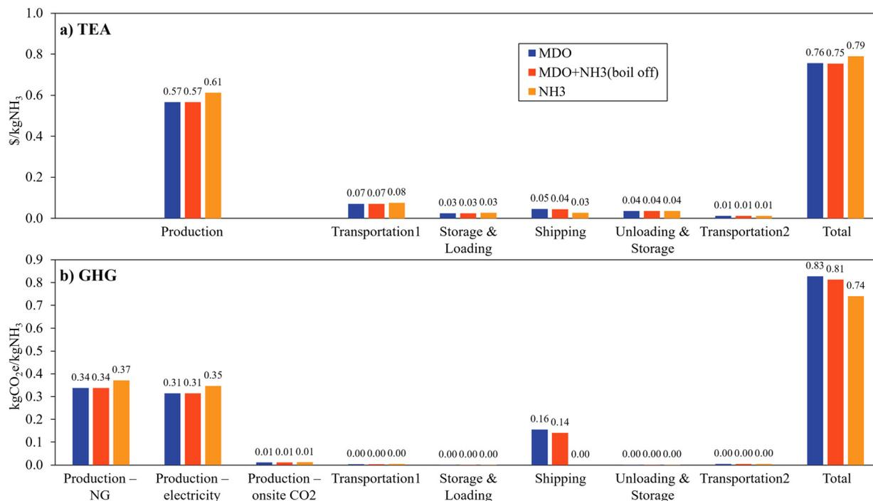
Fig. 6 Effects of shipping fuel option on (a) LCOA and (b) GHG emission (U.S. to Japan, ATR-CCS-OC, grid electricity use, no reconversion to H<sub>2</sub>, 100 tonnes NH<sub>3</sub> per h delivery).
