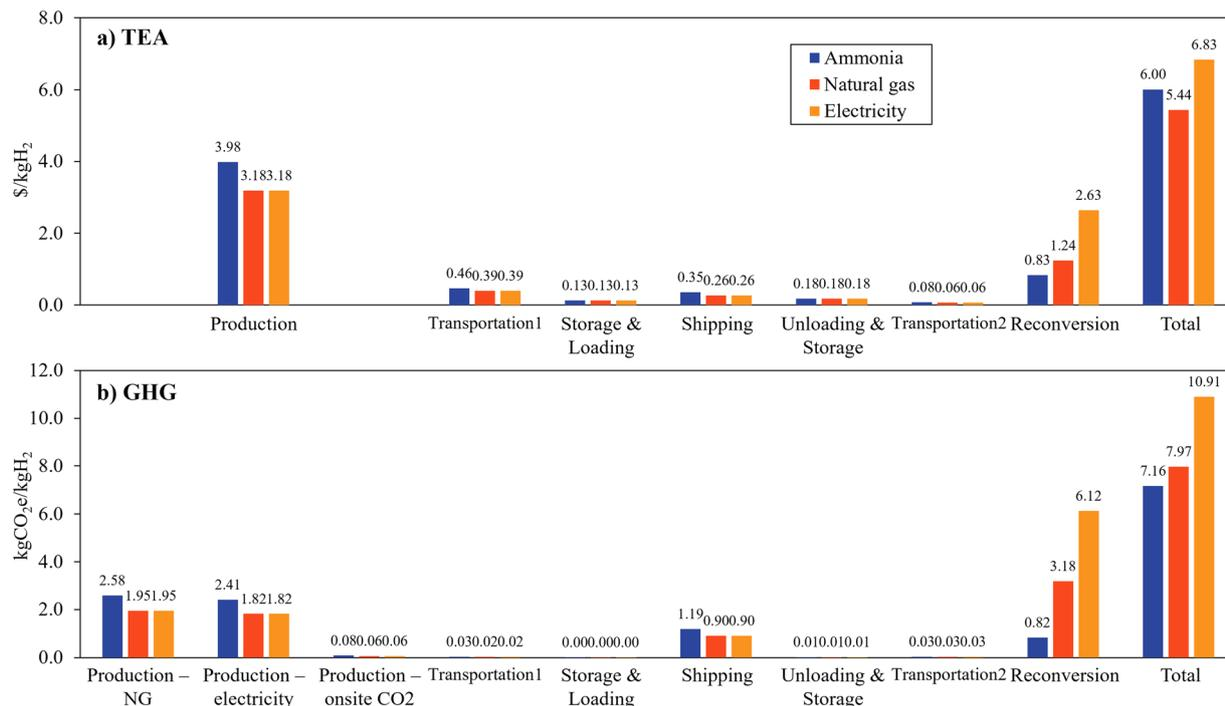
Fig. 7 Effects of reconversion fuel option on (a) LCOH and (b) GHG emission (U.S. to Japan, ATR-CCS-OC, grid electricity use, MDO for shipping fuel, 17.2 tonnes H<sub>2</sub> per h delivery).
