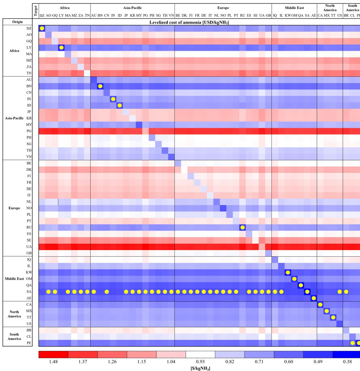
Fig. 12 Blue NH<sub>3</sub> inter-country cost [\$ per kgNH<sub>3</sub>]. Note that, EG, NA, NG, KZ, TM, UZ, AZ, CZ, BO, TR, IR, AR, and VE have been excluded for clearer visualization due to their out-ranged FCR, source availability, and their landlocked location. The diagonal line represents the domestic production cases. Yellow dot indicates the lowest origin country option for the corresponding target country.
