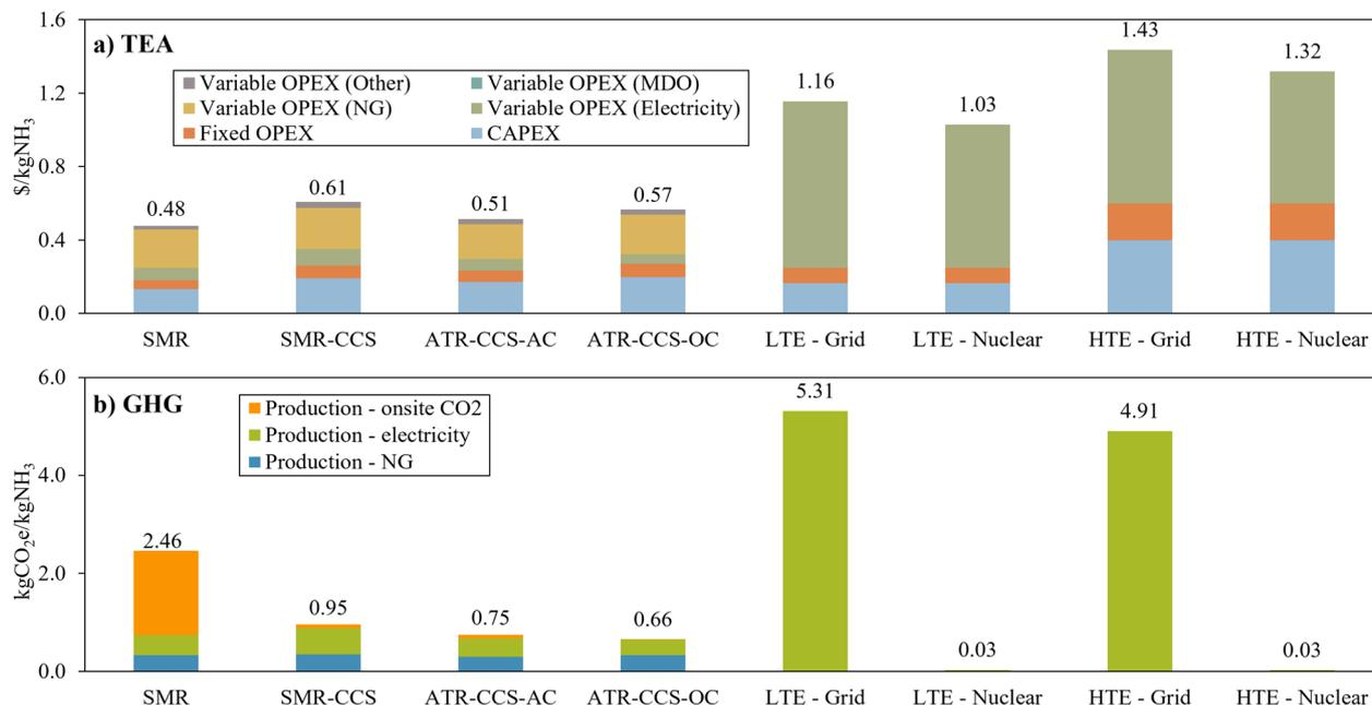
Fig. 5 (a) LCOA and (b) life cycle GHG emission of different NH<sub>3</sub> production technologies (US production, 100 tonnes NH<sub>3</sub> per h production).
