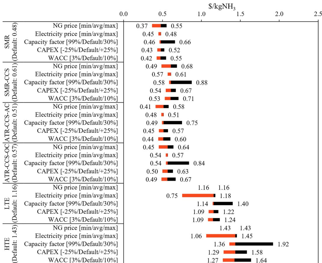
Fig. 16 Sensitivity of key TEA parameters to LCOA. Assumed US production and 100 tonnes NH<sub>3</sub> per h scenario.
