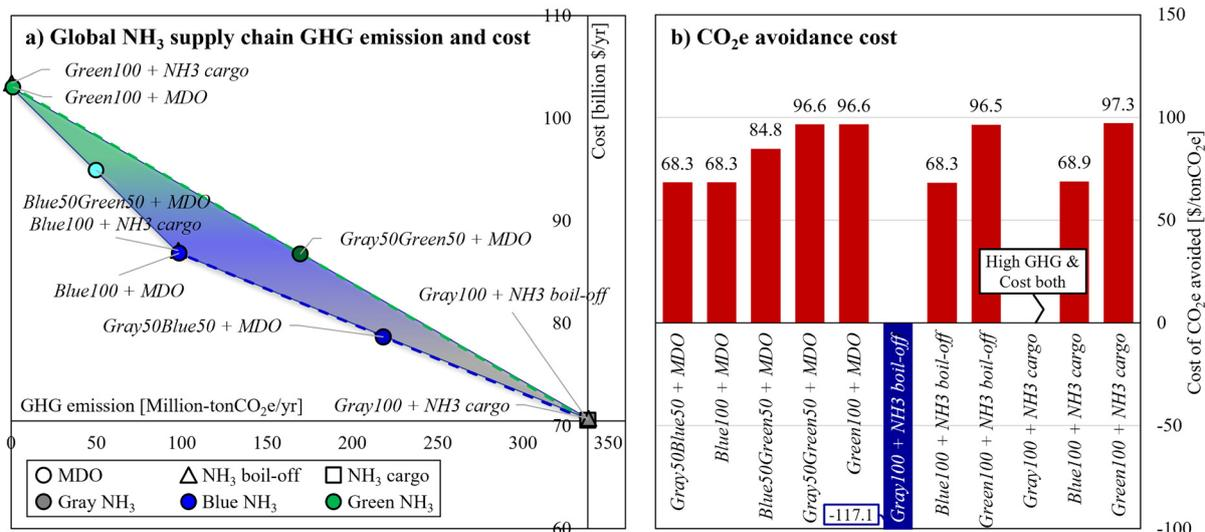
Fig. 19 Impact of decarbonization pathways on global ammonia supply chain's (a) total GHG emission and cost and (b) CO<sub>2</sub>e avoidance cost. (Note for (a): the baseline point represents the current configuration's GHG emission (338.0 million tonneCO<sub>2</sub>e per year) and cost (\$70.6 billion per year). The colored triangle indicates the decarbonization frontier achievable with these options.)
