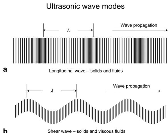
Fig. 7 Ultrasound wave modes classification: (a) compressional (longitudinal) wave, whose particle motion is parallel to the wave propagation direction and (b) shear wave, whose particle motion is perpendicular to the wave propagation.
