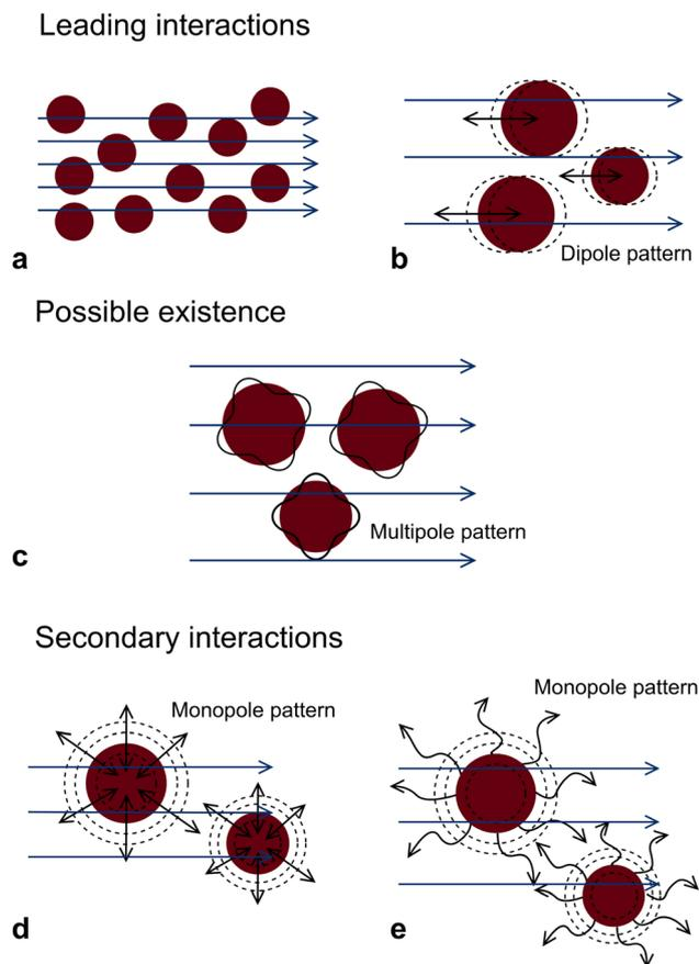
Fig. 9 Leading interaction mechanisms between ultrasonic waves and a suspended particle in a concentrated slurry.<sup>40</sup> (a) Material substitution; (b) density contrast; (c) multipole particle resonance (strong when incident wave length matches resonance). Secondary mechanisms: (d) compressibility contrast; (e) thermal contrast.
