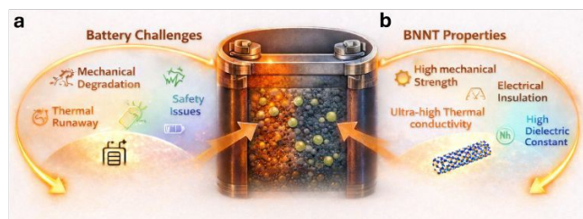
Figure 1. BNNT-enabled solutions to key challenges in lithium-based batteries. (a) Major failure modes and performance limitations in rechargeable lithium batteries include mechanical degradation, thermal runaway, electrolyte instability, safety concerns, and limited cycle life. (b) Intrinsic properties of BNNTs make them uniquely suited for battery engineering, which includes ultra-high thermal conductivity, high mechanical strength, electrical insulator, and high dielectric constant.
