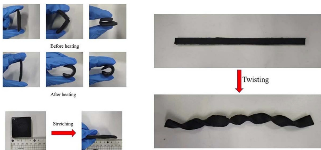
Fig. 17 Thermal-induced flexibility experimental results. Reproduced with permission from ref. 147. Copyright 2024, Elsevier.
