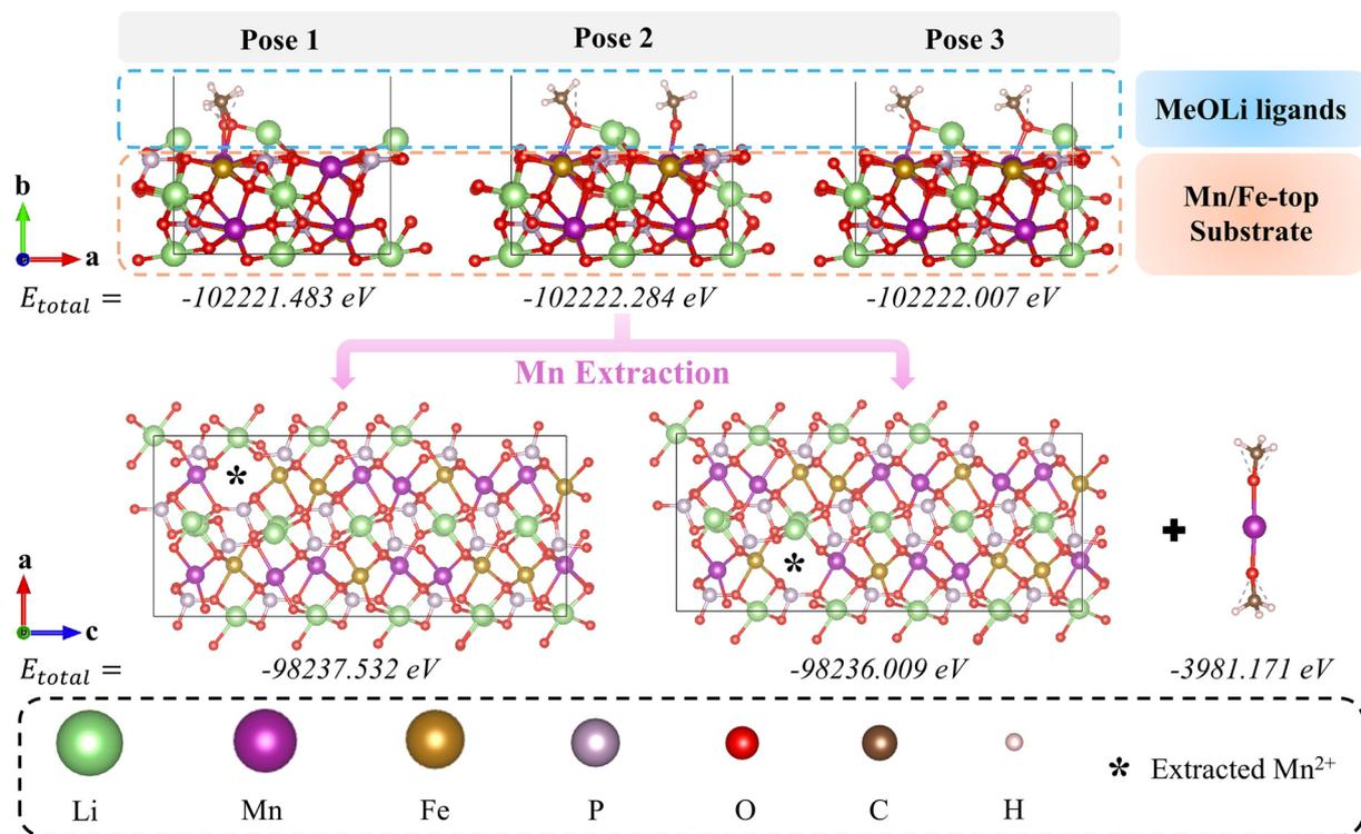
**Fig. 5** MeOLI-assisted  $\text{Mn}^{2+}$  dissolution process investigated by DFT. Three types of MeOLI attaching configurations on the  $\text{LiMn}_{0.6}\text{Fe}_{0.4}\text{PO}_4$  cathode surface were enumerated. Afterwards,  $\text{Mn}^{2+}$  from two different types of sites were extracted from the surface together with the  $\text{MeO}^-$  anions, forming  $\text{Mn}(\text{MeO})_2$ .
