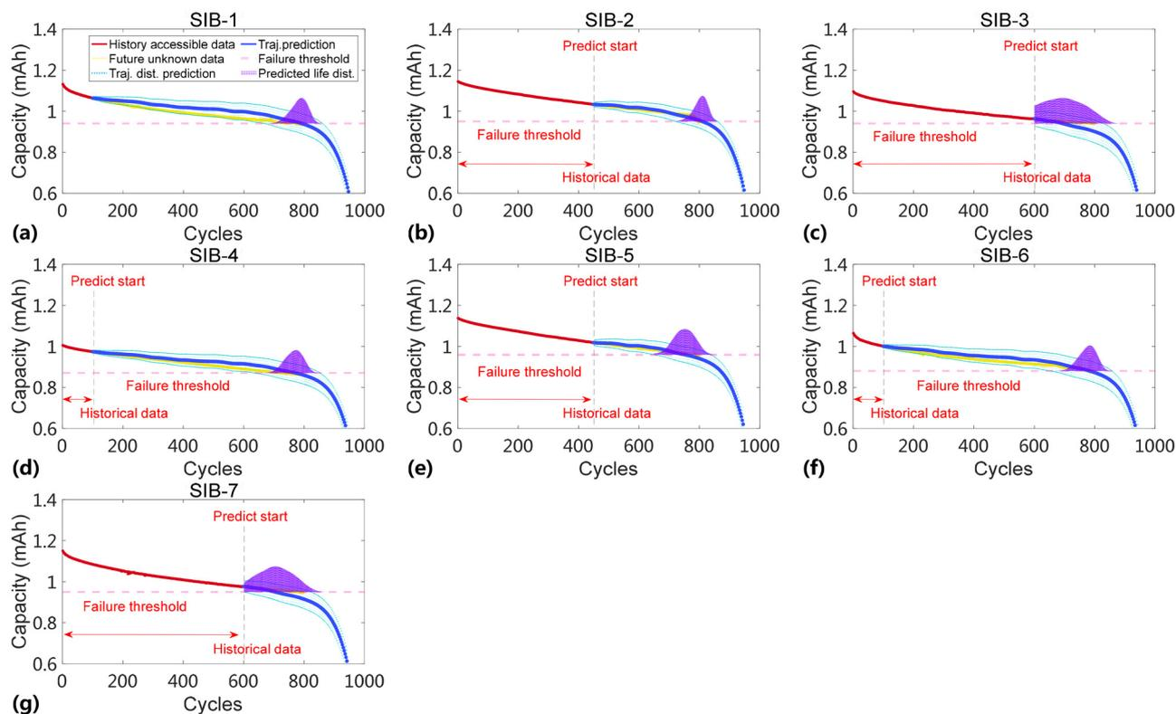
Fig. 6 The capacity prediction results for sodium-ion batteries.
