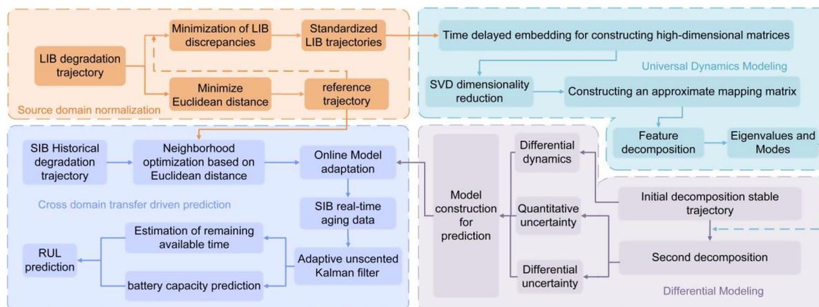
Fig. 3 Cross-battery type RUL prediction framework.
