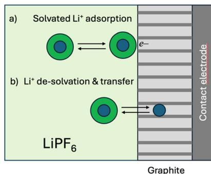
**Fig. 3** (a) Schematic representation of the adsorption of a solvated lithium cation on the negatively charged surface of graphite. (b) Schematic transfer of a lithium cation from the electrolyte solution, where it exists in a solvated state, to graphite, where it becomes a bare cation. By definition, the partially lithiated graphite phase remains electrically neutral overall as a result of the electrical charging of the graphite.
