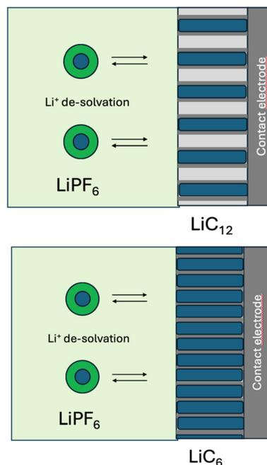
**Fig. 4** Schematic reaction between solvated lithium cation and the solid phase  $\text{LiC}_{12}$  (top) and  $\text{LiC}_6$  (bottom). The blue represents the graphite sheets filled to form a solid phase.
