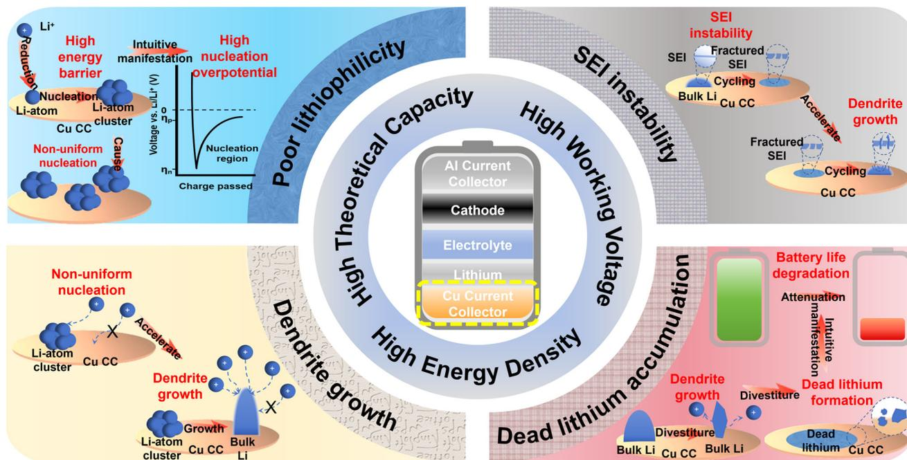
Fig. 1 Advantages of lithium metal batteries and issues when using electroplated copper foil as a lithium anode.
