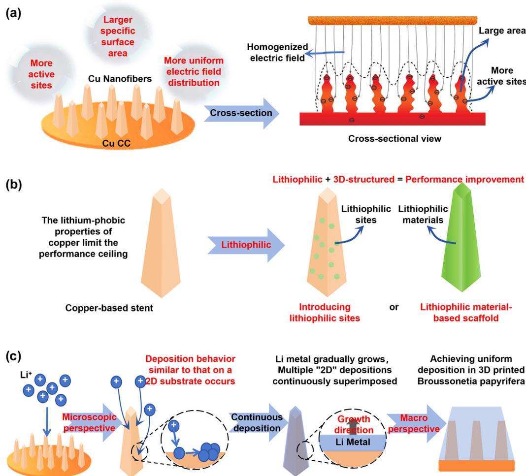
Fig. 6 (a) Schematic diagrams of 3D scaffold structures, along with its cross-sectional view. Copyright © 2015, C. Yang et al.<sup>114</sup> (b) Schematic diagram of lithiophilic scaffold construction. (c) Schematic diagram of uniform Li deposition induced by scaffold structure.
