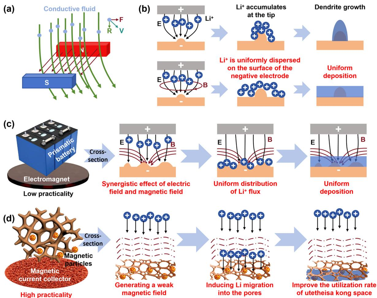
**Fig. 9** (a) Schematic diagrams of magnetohydrodynamics. (b) Schematic diagram of the inductive effect of magnetic field on lithium ions. (c) Introduction of external magnetic field and its mechanism of action. (d) Construction of the magnetic current collector and its mechanism of action.
