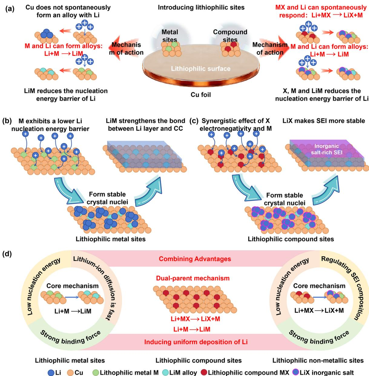
**Fig. 4** (a) Schematic diagram of the lithiophilic mechanisms at two types of sites. Schematic diagram of (b) the influence of lithiophilic metal sites and (c) lithiophilic compound sites on lithium deposition behavior. (d) Characteristics of various lithium-affinity mechanisms.
