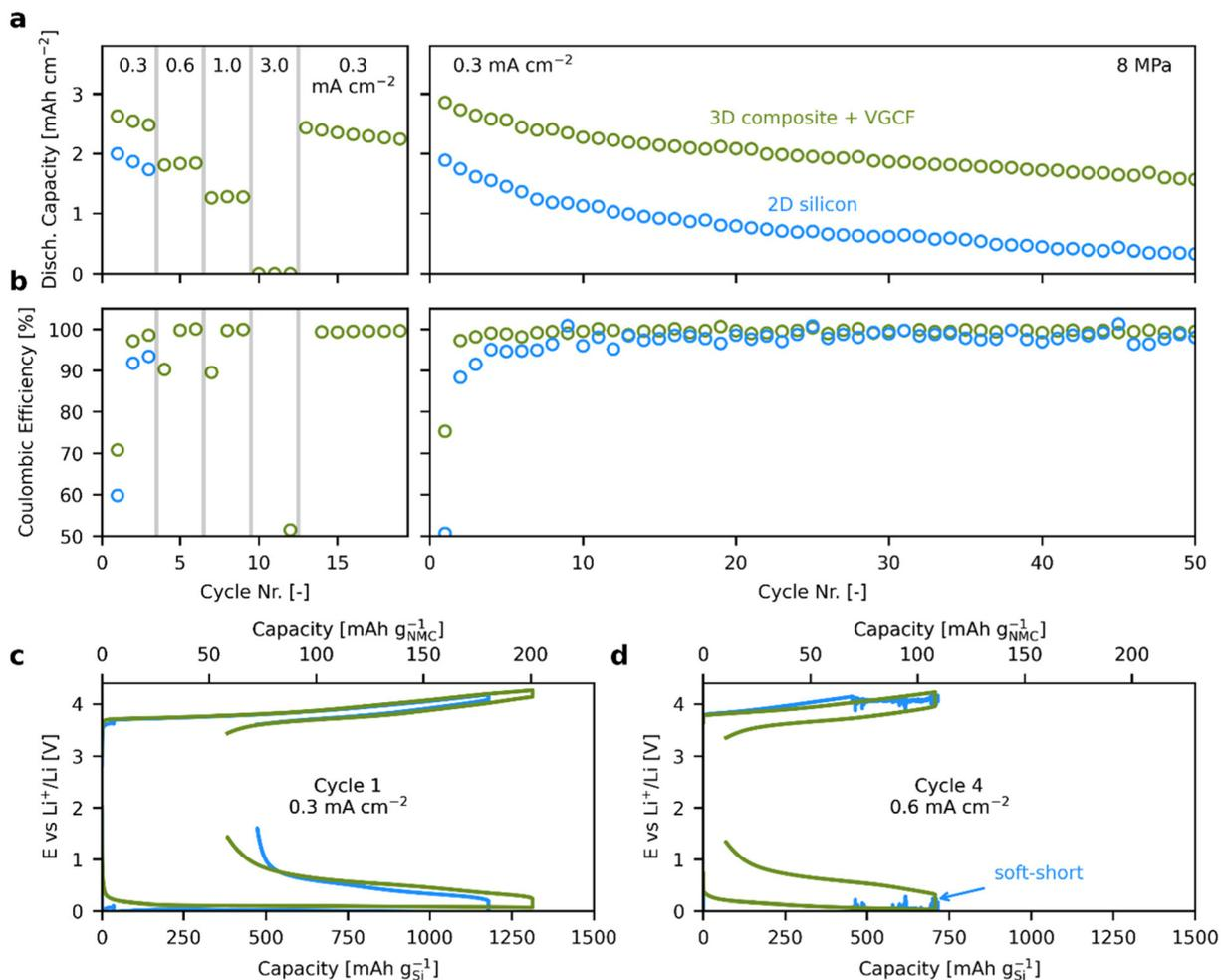
**Fig. 4** (a) Discharge capacity and (b) coulombic efficiency of solid-state cells with NMC811 positive electrode and 3D silicon composite (light green) or 2D silicon (light blue) negative electrode, cycled under 8 MPa stack pressure at 25 °C. (c and d) Individual potential profiles of the NMC811 positive electrode and the silicon negative electrode in the first cycle and in the fourth cycle, measured in three-electrode full cells with an In/InLi reference electrode.
