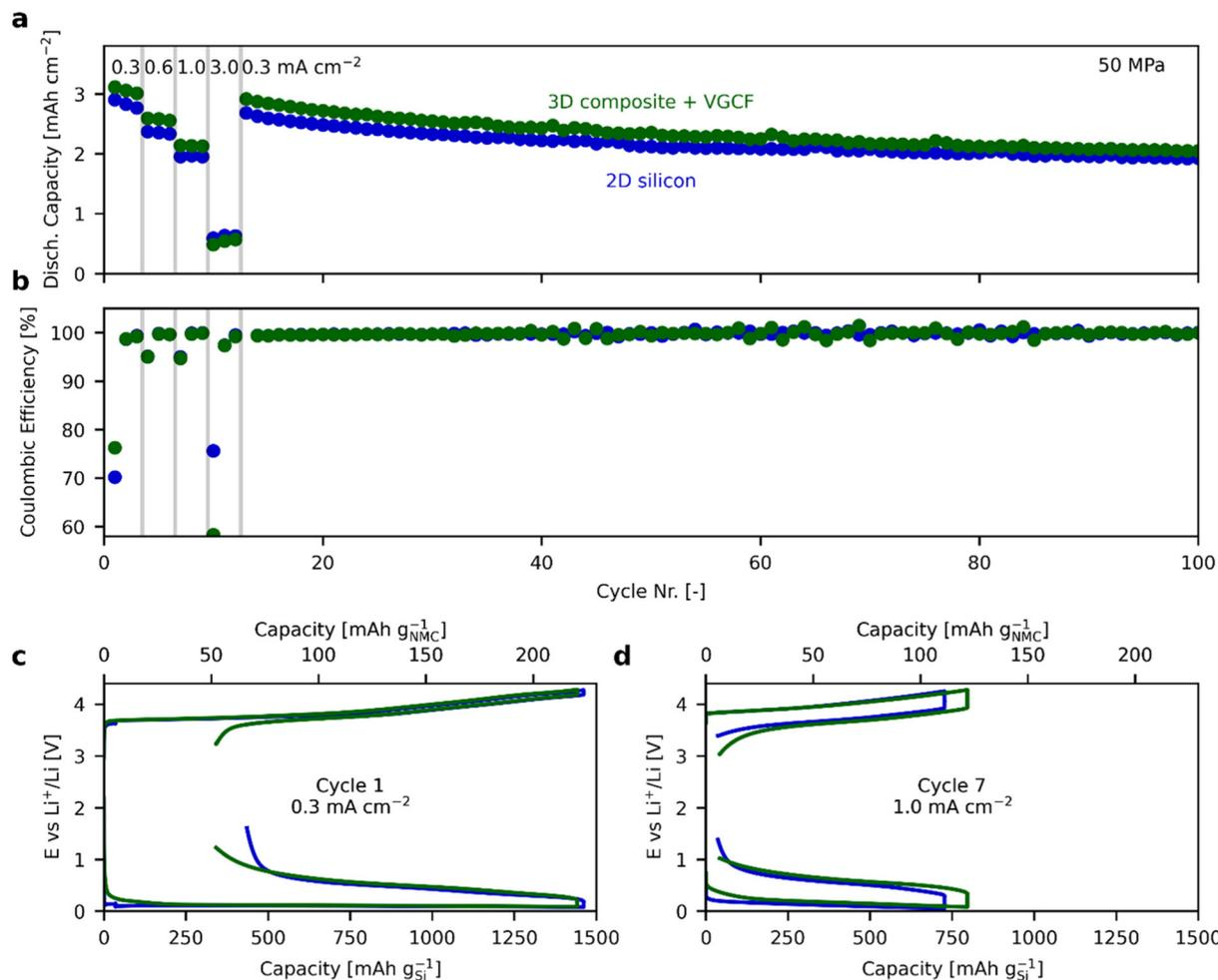
**Fig. 3** (a) Discharge capacity and (b) coulombic efficiency of solid-state cells with NMC811 positive electrode and 3D silicon composite with vapor-grown carbon fibers (green) or 2D silicon (blue) negative electrode, cycled under 50 MPa stack pressure at 25 °C. (c and d) Individual potential profiles of the NMC811 positive electrode and the silicon negative electrode in the first cycle and in the seventh cycle measured in three-electrode full cells with an In/InLi reference electrode.
