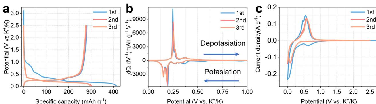
**Fig. 1** The electrochemistry of K metal|1 M KN(SO<sub>2</sub>F<sub>2</sub>)<sub>2</sub> in EC and DEC (1 : 1 in volume)|graphite batteries. (a) The first three galvanostatic discharge–charge cycles at 16 mA g<sup>−1</sup>; (b) the differential capacity of the first three galvanostatic discharge–charge cycles; (c) the first three cyclic voltammetry (CV) profiles at 0.1 mV s<sup>−1</sup>.
