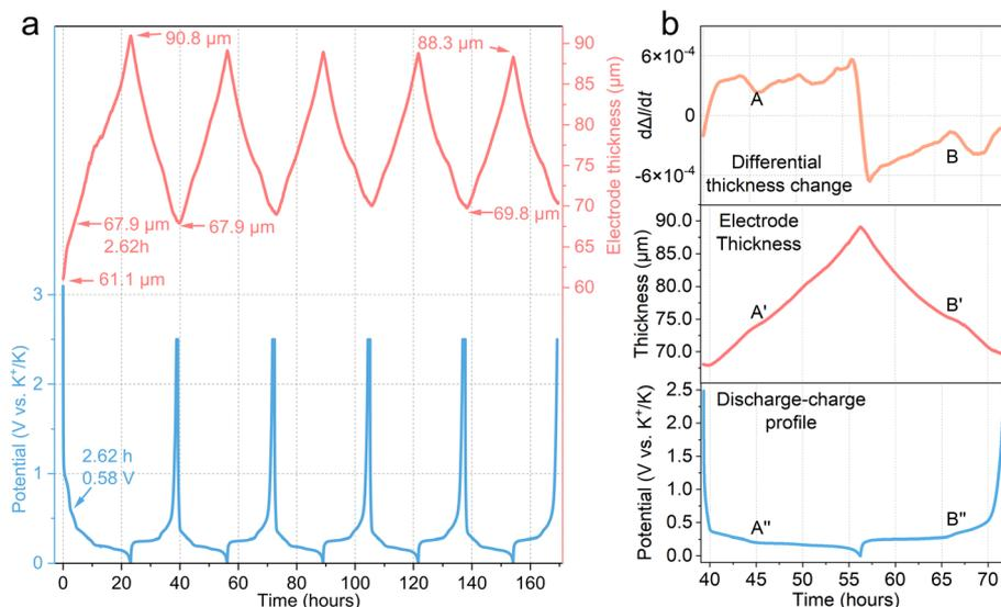
**Fig. 2** *Operando* electrochemical dilatometry analysis. (a) For the first five cycles (in blue) at  $16 \text{ mA g}^{-1}$ , with the change in thickness (in pink). The thickness of the pristine graphite electrode is  $61.1 \mu\text{m}$ ; (b) the change of the electrode thickness and its differential change in the second cycle.
