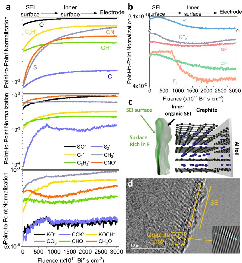
**Fig. 6** *Ex situ* ToF-SIMS depth profiling (using  $\text{Bi}^+$  primary ion beam only) in the graphite electrode (a) for C-containing, O-containing, and S-containing species, and (b) for F-containing species. All the data are point-to-point normalised to total counts; (c) the schematic diagram of the KFSI-derived thin SEI layer on graphite; (d) an *ex situ* TEM image of the cycled graphite after the first cycle.
