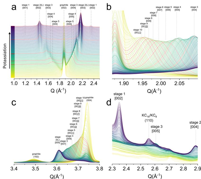
**Fig. 3** Operando synchrotron X-ray diffraction patterns for the first potassiation cycle (a)  $Q$  range from 1.0–2.5 Å<sup>-1</sup>, the highlighted red patterns are K-GICs stage 2–5 and stage 1/stage 2, stage 2L exists between stage 3 and stage 2; (b)  $Q$  range from 1.85 to 2.2 Å<sup>-1</sup>; (c)  $Q$  range from 3.4 to 3.8 Å<sup>-1</sup>; (d)  $Q$  range for the formation of [002] and [003] of stage 2 KC<sub>16</sub>.
