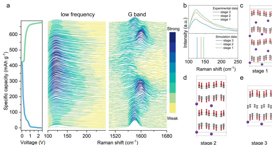
**Fig. 4** (a) *Operando* Raman spectra coloured according to their intensity with the first discharge–charge profile at a constant current of  $16 \text{ mA g}^{-1}$ ; (b) the experimental and simulated data of the low-frequency regions for different K-GICs; (c) the corresponding displacement patterns for the Raman-active modes.
