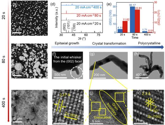
Fig. 4 Mossy deposition growth process. (a-c) SEM morphologies after deposition at 20 mA cm<sup>-2</sup> for (a) 20, (b) 80, and (c) 400 s. (d) XRD patterns at three different stages. (e) Comparative analysis of peak intensities at the three stages. (f-h) TEM images of the (f) whisker initiation, (g) growth, and (h) completion stages. (i-k) HR-TEM images at the (i) left, (j) center and (k) right sides of the black boundary line in (g).
