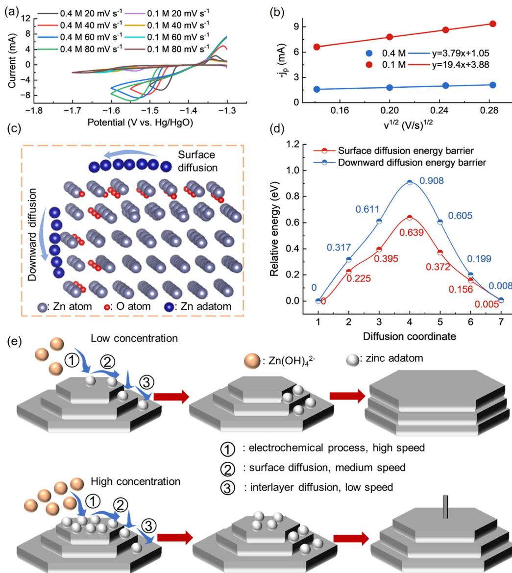
**Fig. 5** Mechanistic analysis of initial whisker formation and the influence of concentration and polarization levels. (a) CV at different concentrations and scan rates. (b) Relationship between peak currents and the square root of scan rates. (c) Surface and interlayer diffusion model with a layer of zinc oxide. (d) Surface and interlayer diffusion energy barriers with a layer of zinc oxide. (e) Schematic diagram of the effect of concentration on the mossy deposition formation.
