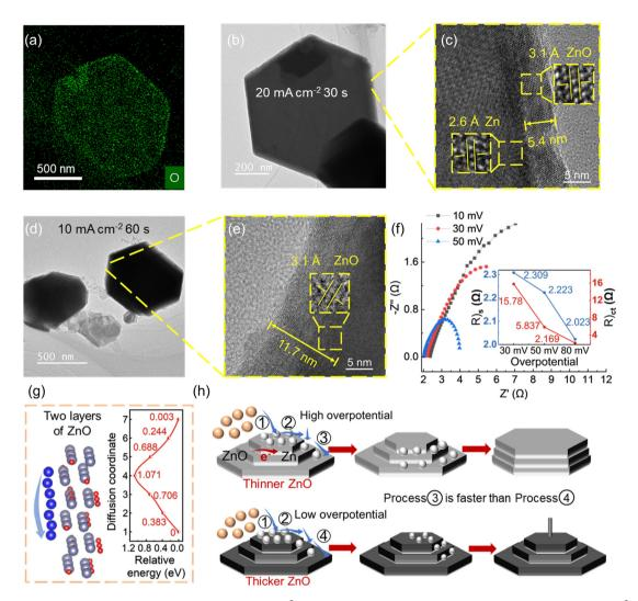
Fig. 6 (a) Oxygen element mapping. (b) TEM image at 20 mA cm<sup>-2</sup> for 30 s. (c) HR-TEM image of (b). (d) TEM image at 10 mA cm<sup>-2</sup> for 60 s. (e) HR-TEM image of (d). (f) EIS at different bias voltages. (g) Interlayer diffusion with two layers of zinc oxide. (h) Schematic diagram of the effect of polarization.
