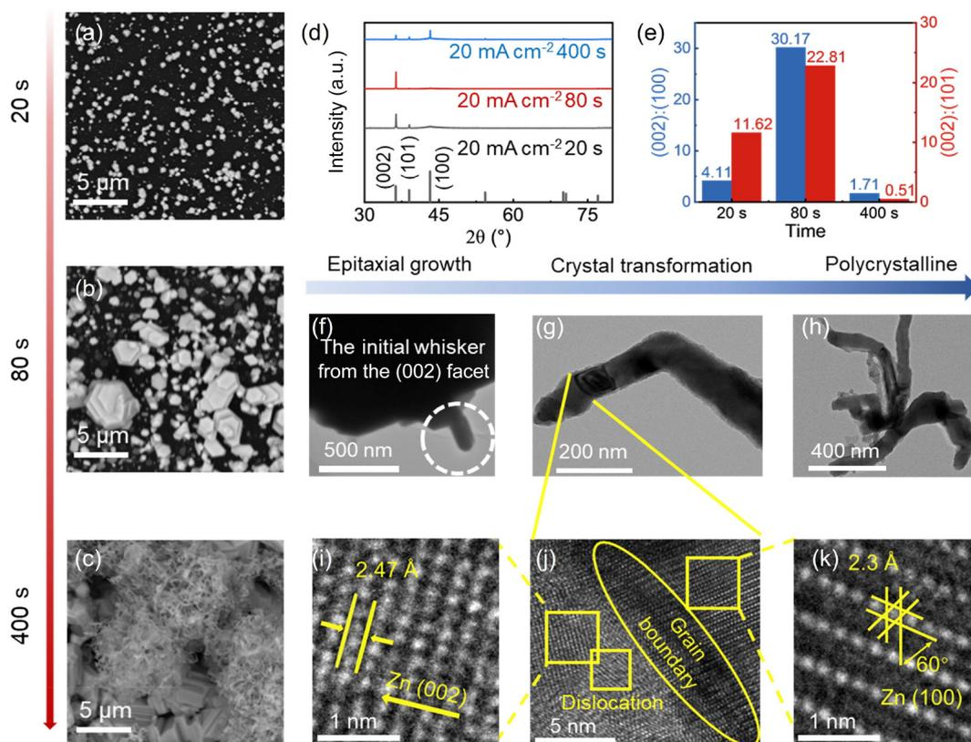
**Fig. 4** Mossy deposition growth process. (a–c) SEM morphologies after deposition at  $20 \text{ mA cm}^{-2}$  for (a) 20, (b) 80, and (c) 400 s. (d) XRD patterns at three different stages. (e) Comparative analysis of peak intensities at the three stages. (f–h) TEM images of the (f) whisker initiation, (g) growth, and (h) completion stages. (i–k) HR-TEM images at the (i) left, (j) center and (k) right sides of the black boundary line in (g).
