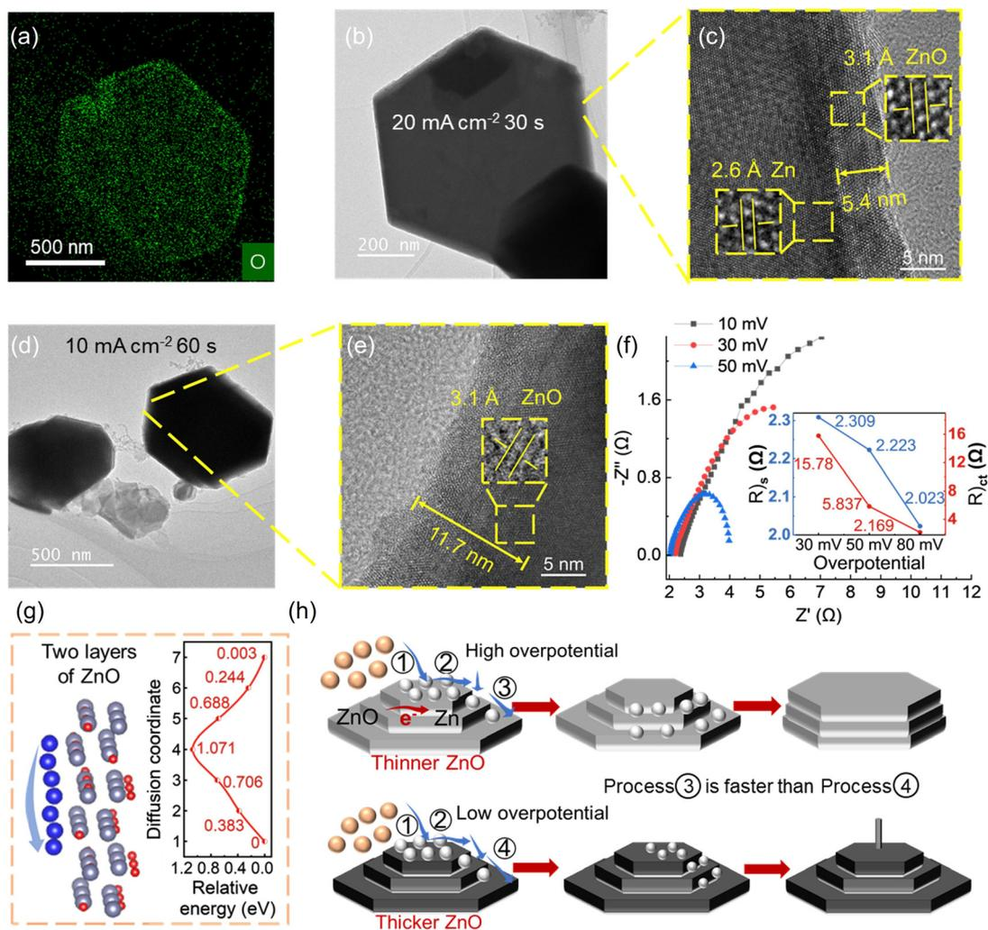
**Fig. 6** (a) Oxygen element mapping. (b) TEM image at  $20 \text{ mA cm}^{-2}$  for 30 s. (c) HR-TEM image of (b). (d) TEM image at  $10 \text{ mA cm}^{-2}$  for 60 s. (e) HR-TEM image of (d). (f) EIS at different bias voltages. (g) Interlayer diffusion with two layers of zinc oxide. (h) Schematic diagram of the effect of polarization.
