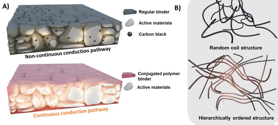
**Fig. 1** (A) Illustration of the classical electrode design (based on PVDF and carbon black) featuring non-continuous conduction pathway, as well as the electrode with conjugated polymer binder featuring continuous conduction pathway. (B) Illustration of conjugated polymer with random coil structure or hierarchically ordered structure with improved crystallinity.
