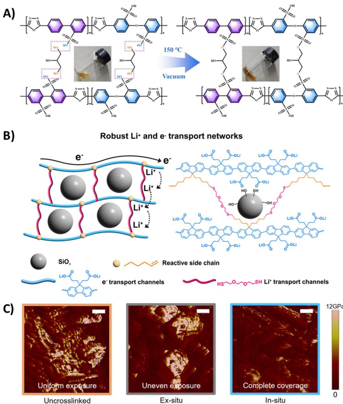
**Fig. 9** (A) Schematic drawing of the crosslinked POD-c-GL binder formed by condensation between LPOD and GL. Reprinted by permission from Wiley, ref. 19, copyright 2024. (B) Architecting an elastic binding network to promote e<sup>-</sup>/Li<sup>+</sup> transport via the proposed *in situ* photo-crosslinking strategy. (C) DMT modulus mappings of the above three binder electrodes. The scale bars represent 300 nm. Reprinted by permission from Cell Press, ref. 78, copyright 2025.
