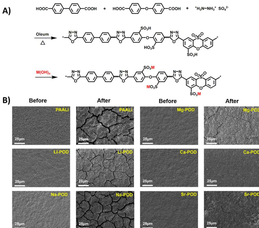
**Fig. 8** (A) Synthesis procedure and structures of  $\text{Mn}^+$ -PODs. (B) SEM images of the Si anodes with PAALi and  $\text{Mn}^+$ -PODs binders before and after 100 cycles at 0.2 C. Reprinted by permission from American Chemical Society, ref. 40. Copyright 2023.
