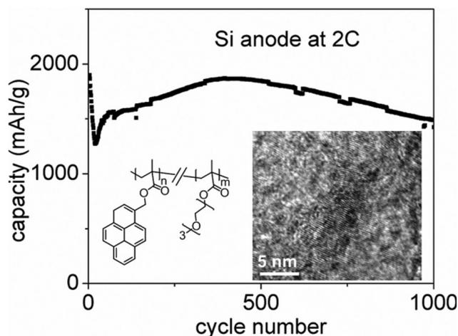
**Fig. 3** Structure of the side chain conducting poly(1-pyrenemethyl methacrylate-co-triethylene oxide methyl ether methacrylate) (PPyE), high-resolution transmission electron microscopy (HRTEM) image of PPyE polymer, and charge (delithiation) capacities of PPyE-based Si electrodes at 2 C rate. Reprinted by permission from American Chemical Society, ref. 50, copyright 2015.
