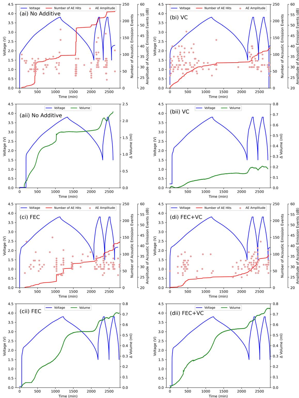
**Fig. 3** Cell cycling data over C/20 formation cycle and C/5 diagnostic cycles. (ai, bi, ci and di) Amplitude of AE hits (red transparent dots) and Cumulative number of AE hits (red line) against cell voltage (blue line). (aii, bii, cii and dii) Change in cell volume against cell voltage. (a) No Additive cell. (b) VC additive cell. (c) FEC additive cell. (d) VC and FEC additive cell.
