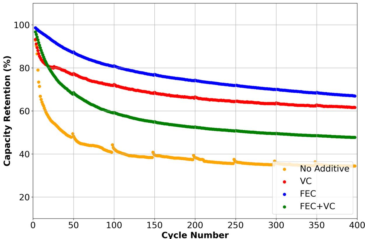
**Fig. 6** Capacity retention for sodium-ion cells with different electrolytes (no additive, VC, FEC, FEC + VC). Cells were cycled at C/3 between 1.5–3.8 V for 400 cycles to assess the impact of electrolyte composition on long-term performance. Electrochemical Cycling repeats for each of these cells using the Novonix are shown in Fig. S20. coulombic Efficiency data is shown in Fig. S21.
