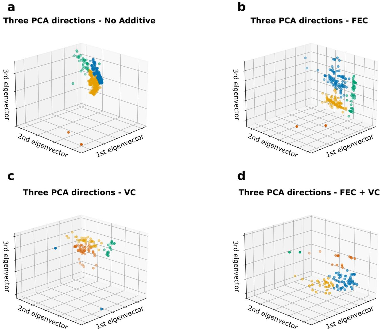
**Fig. 5** 3D plots showing *k*-means clustering results after applying PCA to the multi-dimensional acoustic features dataset. Each colour represents a different cluster. Each subfigure represents the results for each cell containing different electrolyte: (a) no additive (b) FEC (c) VC and (d) FEC + VC.
