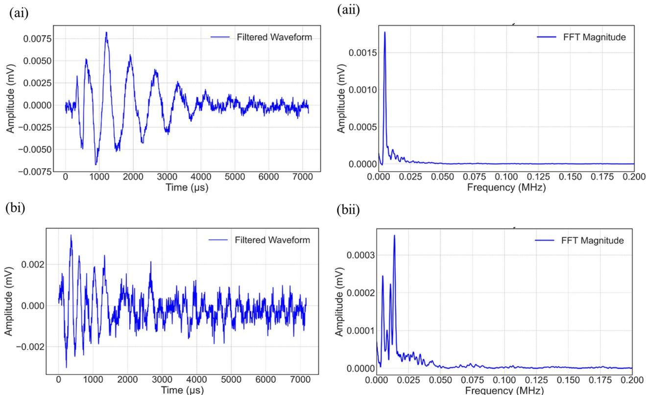
**Fig. 4** Example waveforms in the time domain (ai & bi) and corresponding frequency components (aai & bii). Waveforms are extracted from the cell with no additive. (a) Displays a waveform produced during the first formation cycle and (b) produced later during discharge. Both signals are attributed to gassing within the cell.
