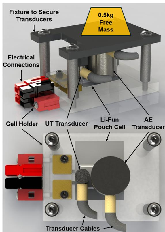
**Fig. 1** Schematic of the experimental set up. Figure outlines the electrical connections to the maccor battery cyclers, the Li-Fun cell, the ultrasonic transducer, acoustic emission transducer, and cell holder.
