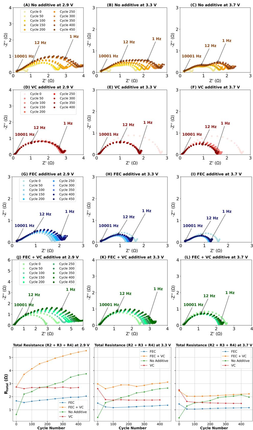
**Fig. 7** Top figure displays EIS Nyquist plots and total fitted resistance ( $R_2 + R_3 + R_4$ ) for sodium-ion cells containing each electrolyte additives (No additive, VC, FEC, and VC + FEC) at 2.9 V, 3.3 V, and 3.7 V over cycling. EIS was measured every 50 cycles up to 450 cycles. Bottom figure shows the evolution of total fitted resistance fitted ( $R_{total}$ ) with the equivalent circuit model (ECM) shown in Fig. S1.
