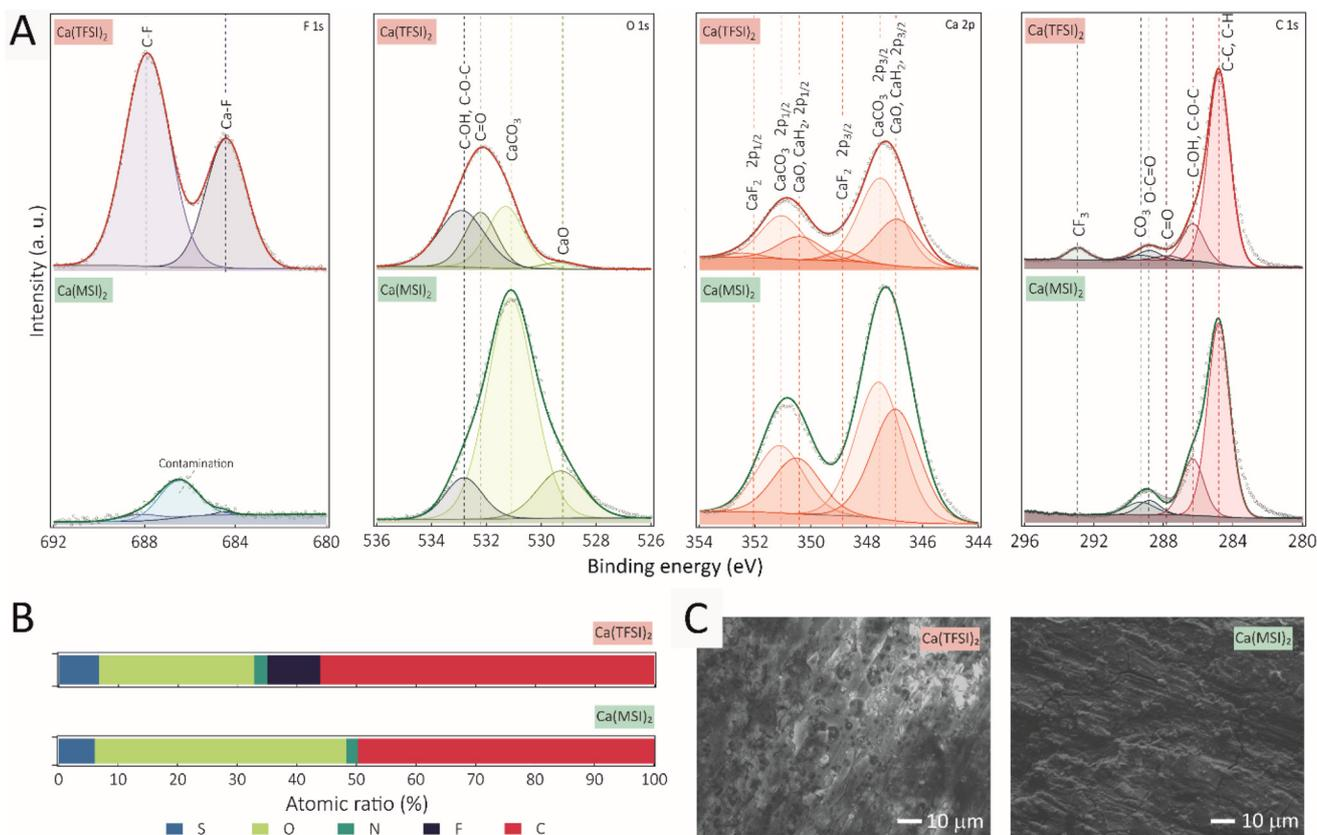
**Fig. 4** (A) XPS profiles, (B) atomic ratio, and (C) SEM images of the SEIs formed on the Ca-electrode after 10 cycles in 0.5 M  $\text{Ca}(\text{MSI})_2$  and  $\text{Ca}(\text{TFSI})_2$  in DMAC electrolytes.
