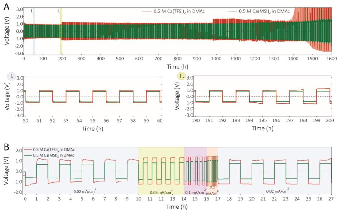
Fig. 3 (A) Cyclic stability at 0.02 mA cm<sup>-2</sup> and (B) rate capability of Ca/Ca symmetric cells in 0.5 M Ca(MSI)<sub>2</sub> and Ca(TFSI)<sub>2</sub> in DMAc electrolytes.
