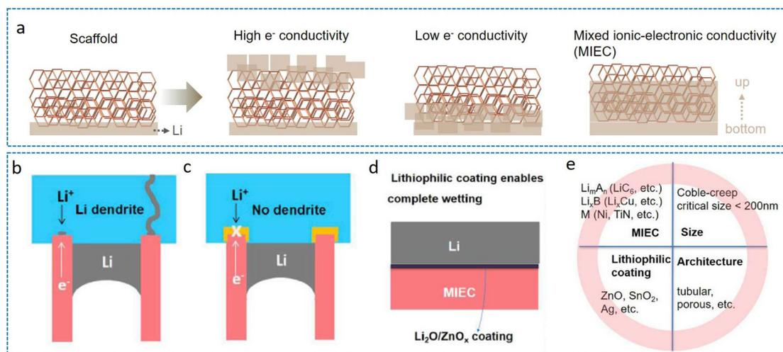
**Fig. 5** (a) Schematic illustration of the influence of scaffold materials on lithium deposition behavior. (b and c) Working mechanisms of MIEC (b) without or with (c) ELI in 3D LMA. (d) The great wetting performances with the existence of a lithiophilic coating. (e) The design details with respect to the 3D porous MIEC/ELI structures.<sup>59</sup> Reproduced with permission from Elsevier, copyright 2020.
