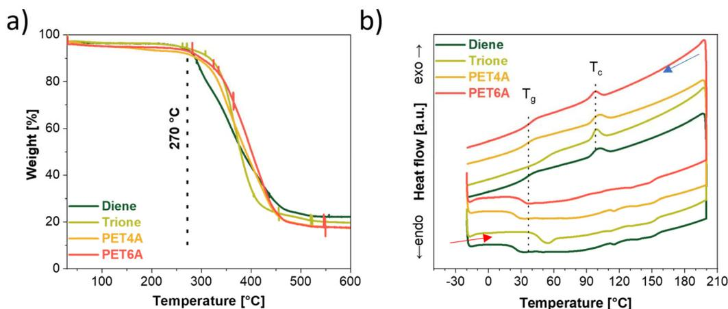
Fig. 5 (a) TGA and (b) DSC of dry diene-, trione-, PET4A- and PET6A-based SIPEs (heating rate of 5 °C min<sup>-1</sup>, inert N<sub>2</sub> atmosphere, the DSC was performed by two cooling and heating cycles between -20 and 200 °C).
