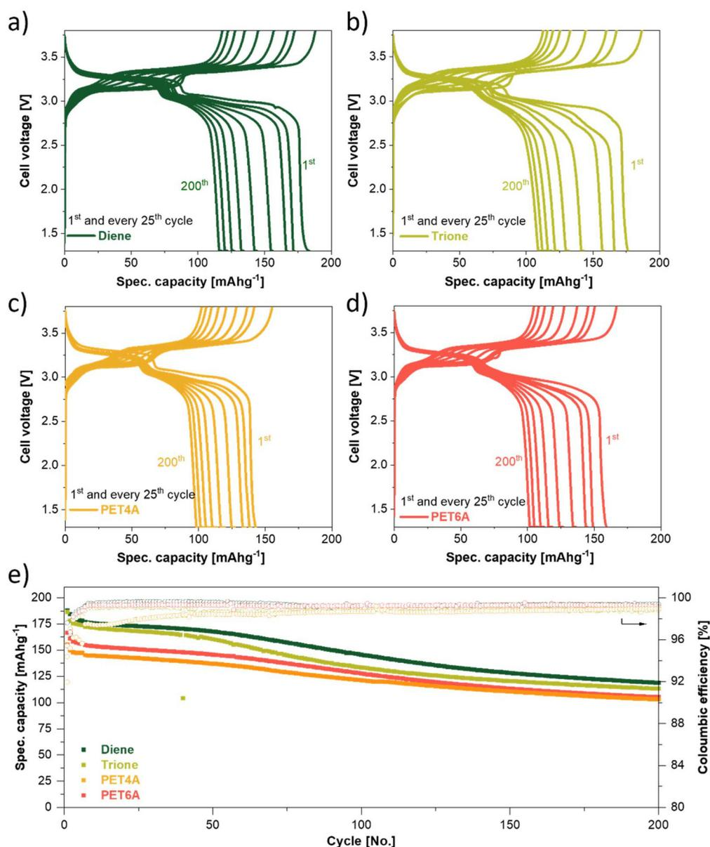
**Fig. 8** Voltage profile of Na|SIPE|PW cells, containing (a) diene-, (b) trione-, (c) PET4A- and (d) PET6A-SIPE and the corresponding (e) cycling performance (capacity vs. cycle number and the corresponding coulombic efficiency). Galvanostatic cycling tests are performed at C/50 (1<sup>st</sup> cycle), followed by C/20 (5 cycles) and C/10 until failure between 3.8 V and 1.3 V. All measurements were performed at 40 °C. The SIPEs contain 50 wt.% of EC:DMC:FEC.
