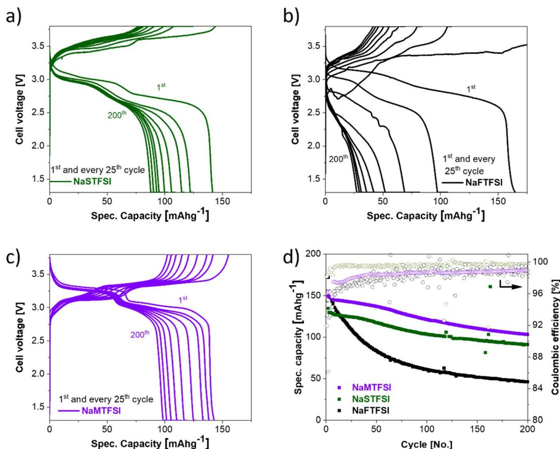
**Fig. 3** Voltage profile of Na||PW cells using (a) NaSTFSI-, (b) NaFTFSI- or (c) NaMTFSI-SIPEs, and the corresponding (d) specific capacity and Coulombic efficiency. In all SIPEs, EC:DMC:FEC (49:49:2 vol.%) is incorporated, serving as molecular transporter. The galvanostatic cycling tests are conducted at a C-rate of C/50 in the first cycle, followed by 5 cycles at C/20, and continuous cycling at C/10 between 3.8 V and 1.3 V at 40 °C.
