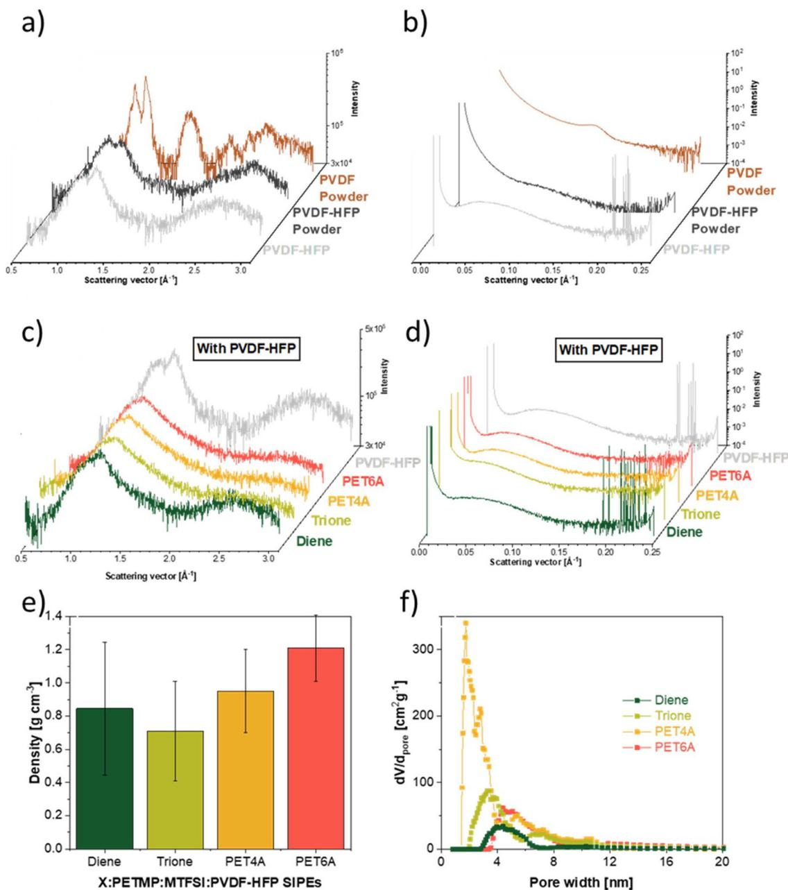
Fig. 6 (a) WAXS and (b) SAXS patterns of commercial PVDF and PVDF-HFP powders, and PVDF-HFP membrane. (c) WAXS and (d) SAXS patterns, (e) density and (f) calculated pore size of the dry diene-, trione-, PET4A- and PET6A-SIPes blended with PVDF-HFP.
