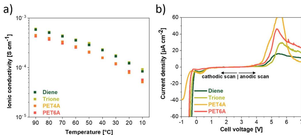
Fig. 7 (a) Temperature-dependent ionic conductivity, and (b) electrochemical stability window (Al|SIPE|Na; scan rate: 30  $\mu\text{V s}^{-1}$ ; temperature: 40  $^{\circ}\text{C}$ ) of the diene-, trione-, PET4A- and PET6A-SIPE containing 50 wt.% of molecular transporters (EC:DMC:FEC).
