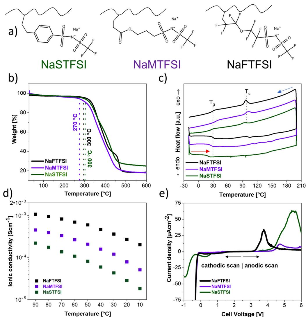
**Fig. 1** (a) Chemical structure of the studied SSMs. (b) TGA and (c) DSC (heating rate of 5 °C min<sup>-1</sup>, N<sub>2</sub> atmosphere for both experiments) data of NaSTFSI- (green), NaMTFSI- (purple) and NaFTFSI (black)-dry SIPEs. (d) Temperature-dependent ionic conductivity and (e) electrochemical stability window (Na||SIPE||Al, scan rate of 30 μV s<sup>-1</sup> at 40 °C) of NaSTFSI-, NaMTFSI- and NaFTFSI-based SIPEs containing 50 wt.% of EC:DMC:FEC.
