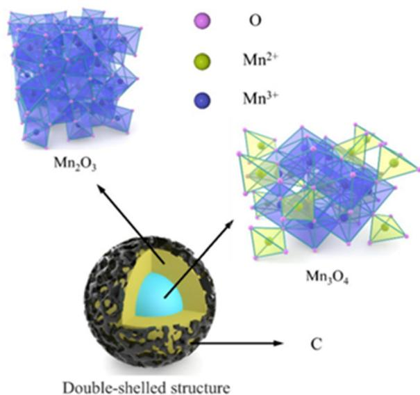
**Fig. 5** A ternary anode of C,  $\text{Mn}_2\text{O}_3$  and  $\text{Mn}_3\text{O}_4$ . Reproduced with permission.<sup>119</sup> Copyright 2024, Springer Nature.
