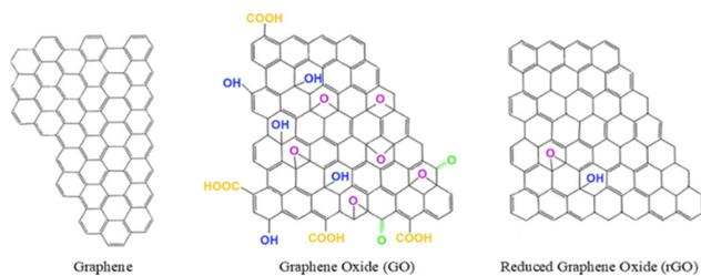
Fig. 7 Structures of graphene, GO and rGO. Reproduced with permission.<sup>132</sup> Copyright 2015, Royal Society of Chemistry.
