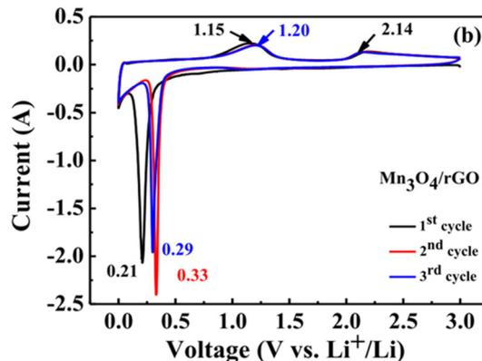
**Fig. 11** Cyclic voltammograms of  $\text{Mn}_3\text{O}_4/\text{rGO}$  anode at a scan rate of  $0.1 \text{ mV s}^{-1}$  in a potential range of 0.01–3 V. Working electrode = Active material: Super P:LiOH:PAA in a mass ratio of 80:10:5:5. Counter electrode = Li foil. Electrolyte = 1 M  $\text{LiPF}_6$  in 1:1 EC and DEC. Reproduced with permission.<sup>84</sup> Copyright 2020, Elsevier.
