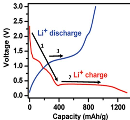
**Fig. 8** Charge and discharge curve of the Mn<sub>3</sub>O<sub>4</sub>/rGO anode for the first cycle at a current density of 40 mA g<sup>-1</sup> in a potential range of 0.1–3 V vs. Li<sup>+</sup>/Li. Working electrode = Mn<sub>3</sub>O<sub>4</sub>/rGO : carbon black : PVDF in a mass ratio 80 : 10 : 10. Counter electrode = Li foil. Electrolyte = 1 M LiPF<sub>6</sub> in 1 : 1 EC and DEC. Reproduced with permission.<sup>50</sup> Copyright 2010, American Chemical Society.
