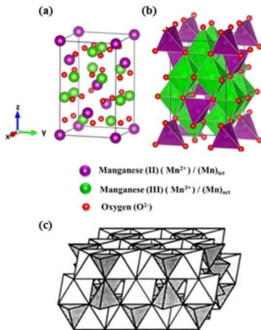
Fig. 3 Structural models of Mn<sub>3</sub>O<sub>4</sub> (a) arrangement of atoms in one unit cell and (b) arrangement of tetrahedra and octahedra in one unit cell. Reproduced with permission.<sup>118</sup> Copyright 2018, Springer Nature. (c) Spinel type structure consisting of MnO<sub>6</sub> octahedra (white) and MnO<sub>4</sub> tetrahedra (grey). Reproduced with permission.<sup>51</sup> Copyright 2011, John Wiley and Sons.
