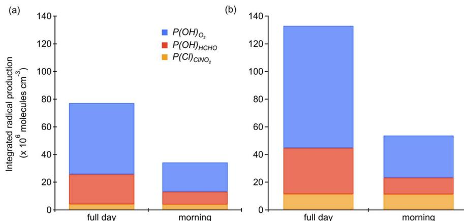
Fig. 5 Integrated ground-level radical production during the HaliFAQS campaign for three radical sources:  $P(\text{HO}_x)$  from reaction of  $\text{O}(^1\text{D})$  from  $\text{O}_3$  photolysis with water (blue),  $P(\text{HO}_x)$  from diurnally averaged HCHO photolysis (red–orange), and  $P(\text{Cl})$  from predicted  $\text{ClNO}_2$  photolysis (yellow–orange) for (a) June 13 and (b) June 18 showing radical contributions for both the full day and the morning (06:00–12:00).
