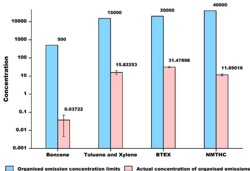
Fig. 2 Comparison of the concentrations (in logarithmic value) of VOCs from the organized emission group and emission standard (DB42/1539–2019, China).<sup>25</sup>
