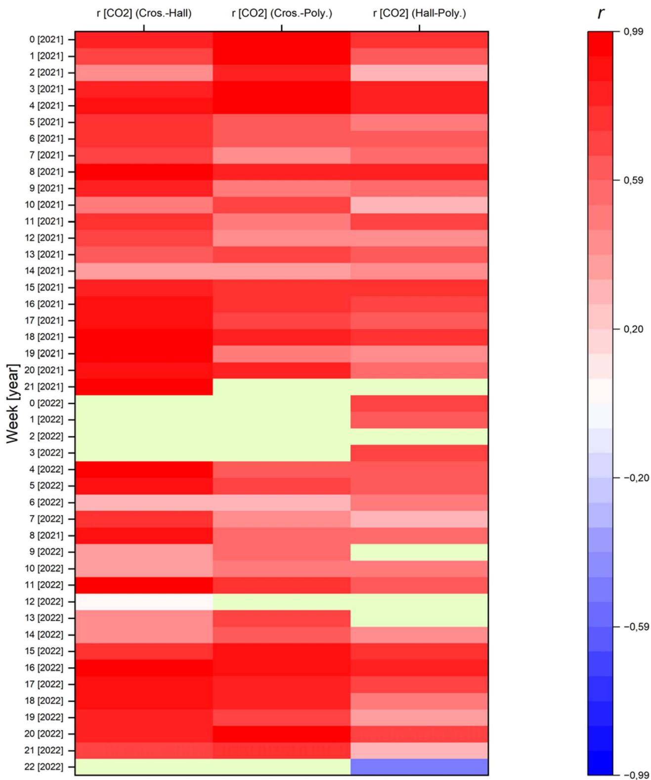
Fig. 10 Correlations between CO<sub>2</sub> concentrations in the indoor rooms. Correlations that are not significant ( $p > 0.01$ ) are coloured light green.
