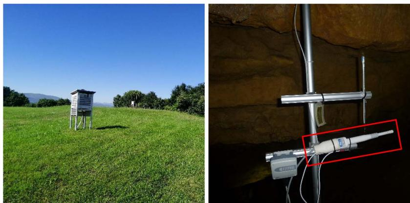
Fig. 2 Measurement stations from the exterior (left) and the mid-section of the Hall (right), as examples, with CO<sub>2</sub> and air temperature sensors marked in red.
