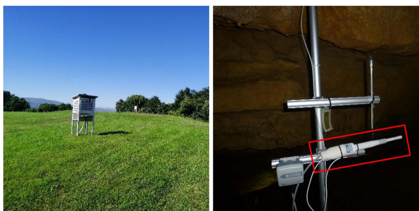
Fig. 2 Measurement stations from the exterior (left) and the mid-section of the Hall (right), as examples, with CO 2 and air temperature sensors marked in red.
