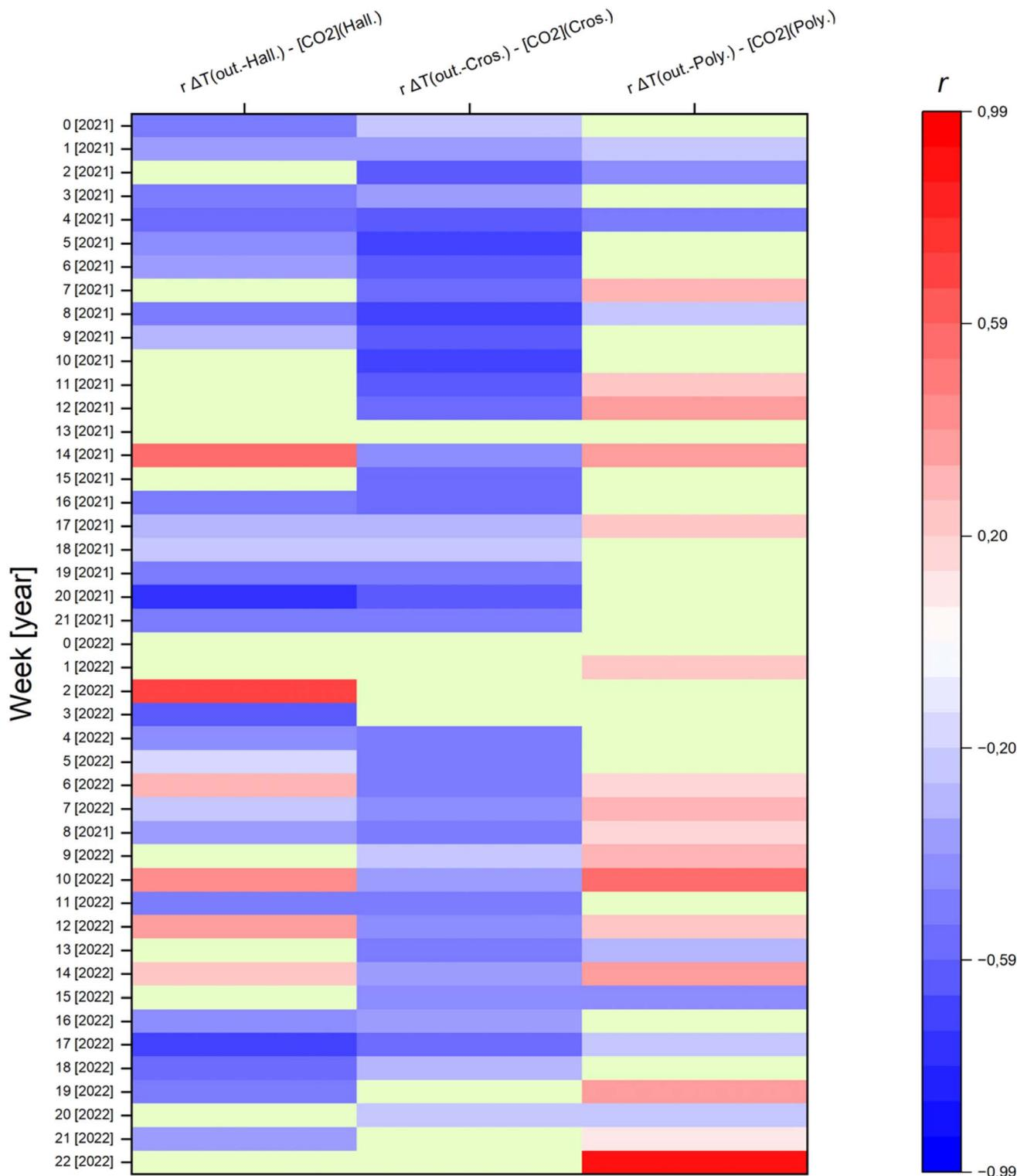
Fig. 11 Correlations between indoor/outdoor air temperature gradients and indoor CO<sub>2</sub> concentrations. Correlations that are not significant ( $p > 0.01$ ) are coloured light green.
