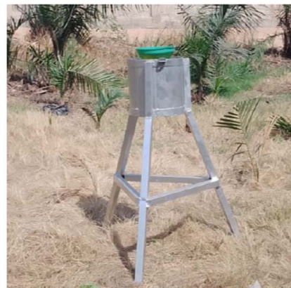
Fig. 2 (a) A 3D schematic design of the rainwater sampler and (b) mounted rainwater sampler at the Sokoban wood village in Kumasi, Ghana.
