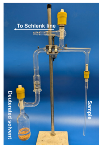
Fig. 13 Vacuum transfer apparatus for condensation of deuterated solvents onto crystalline solid-samples. The NMR tube containing the sample is placed inside a dewar containing a suitable cryogen.
