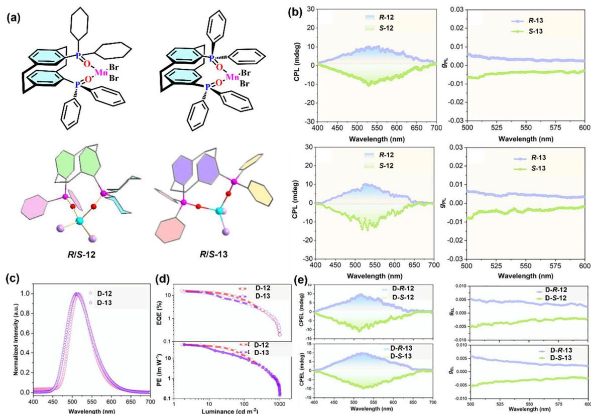
**Fig. 8** (a) Molecular and single-crystal structures, (b) CPL spectra and  $g_{\text{PL}}$  – wavelength curves of the *R/S*-12 and *R/S*-13 enantiomers. (c) EL spectra and (d) EQE–PE–luminance curves of OLEDs based on racemic 12 and 13 complexes. (e) CPEL spectra and  $g_{\text{EL}}$  – wavelength curves of the CP-OLEDs based on *R/S*-12 and *R/S*-13 enantiomers. Reproduced from ref. 40 with permission from Science China Press and Springer, copyright 2025.
