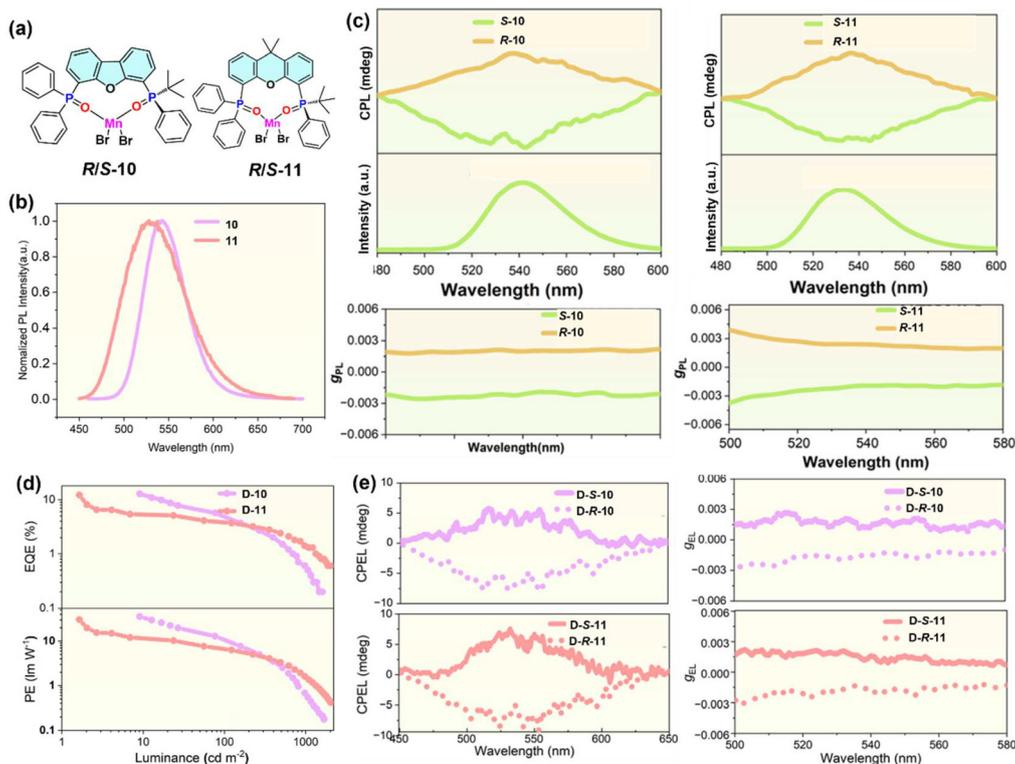
**Fig. 7** (a) Molecular structures, (b) PL spectra, (c) CPL spectra and  $g_{\text{PL}}$  – wavelength curves of the *R/S*-10 and *R/S*-11 enantiomers. (d) External quantum efficiency–luminance curves of *D*-10 and *D*-11 (OLEDs based on *rac*-10 and *rac*-11). (e) CPEL spectra and  $g_{\text{EL}}$  – wavelength curves of *D-R/S*-10 and *D-R/S*-11 (CP-OLEDs based on *R/S*-10 and *R/S*-11 enantiomers). Reproduced from ref. 39 with permission from Wiley-VCH, copyright 2025.
