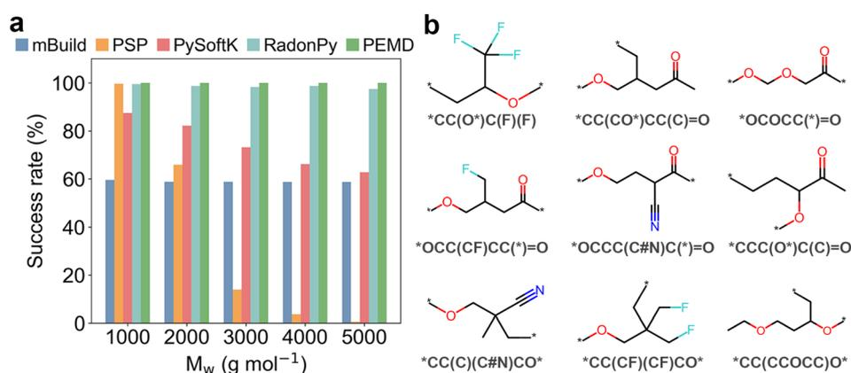
Fig. 8 (a) Success rate of chain generation as a function of molecular weight ( $M_w$ ) comparing multiple tools (mBuild, PSP, PySoftK, RadonPy, and PEMD). (b) Representative monomer units from the benchmark set with their SMILES. \* denotes the connecting sites of the monomers.
