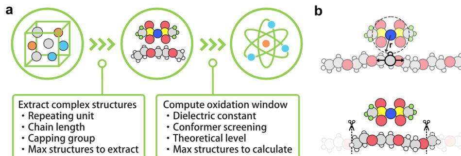
Fig. 6 (a) Automated computational framework for oxidative window. (b) Extraction of ion-polymer complexes from MD trajectories.
