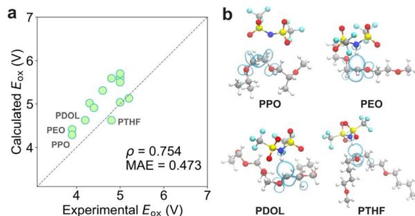
**Fig. 11** (a) Correlation between calculated and experimental oxidation potentials ( $E_{\text{ox}}$ ) at the B3LYP-D3(BJ)/def2-TZVP level of theory. The dashed diagonal line denotes perfect agreement. (b) The spin density distribution (isovalues = 0.003 a.u.) of representative polymer/TFSI<sup>-</sup> complexes.
