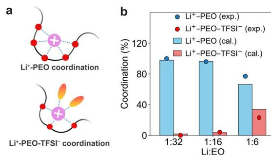
Fig. 10 (a) Schematic first-shell motifs of  $\text{Li}^+$  in PEO electrolytes:  $\text{Li}^+$ -PEO coordination (top) and  $\text{Li}^+$ -PEO-TFSI<sup>-</sup> coordination (bottom). (b) Coordination fraction of  $\text{Li}^+$ -PEO and  $\text{Li}^+$ -PEO-TFSI<sup>-</sup> coordination from experiments and MD simulations at three salt concentrations (Li : EO = 1 : 32, 1 : 16, 1 : 6).
