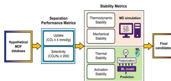
Fig. 7 Workflow for high-throughput computational screening (HTCS) of hMOFs for CO<sub>2</sub> capture as reported in Jiang's work (reproduced with permission from Springer Nature, Copyright© 2023).<sup>70</sup>
