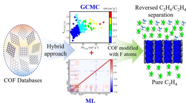
**Fig. 4** The workflow for designing ethane/ethylene separation COF materials as reported in Zhong's work (reproduced with permission from American Chemical Society, Copyright© 2022).<sup>30</sup>
