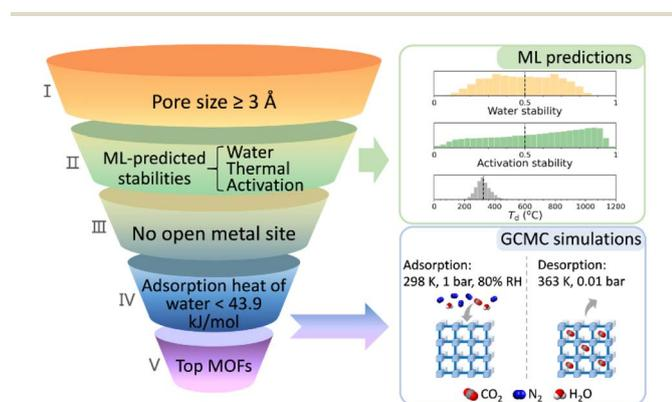
Fig. 6 Workflow for CO<sub>2</sub> capture from wet flue gas using MOFs, as presented in Jiang's work (reproduced with permission from American Chemical Society, Copyright© 2025).<sup>60</sup>
