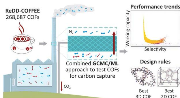
Fig. 5 The workflow for designing CO<sub>2</sub>/N<sub>2</sub> separation COF materials as reported in Van Speybroeck's work (reproduced with permission from American Chemical Society, Copyright© 2024).<sup>66</sup>
