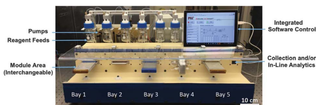
Fig. 7 Plug and play reconfigurable synthesis system, using matching interfaces, modules can be easily and quickly swapped by an operator from a central tubing backbone. Reproduced/modified from Bedard et al. , Science , https://doi.org/10.1126/science.aat0650 [2018], AAAS.
