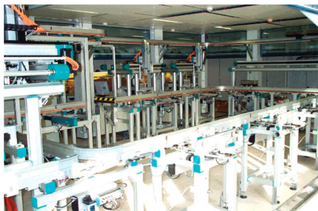
Fig. 3 The Syncar system, glass or plastic vessels travel to different modular stations using a shuttle rail system. Experiment reconfiguration is achieved by changing the order in which the shuttles visit the different modules in software. Reprinted (adapted) with permission from ref. 35 Copyright 2005 American Chemical Society.
