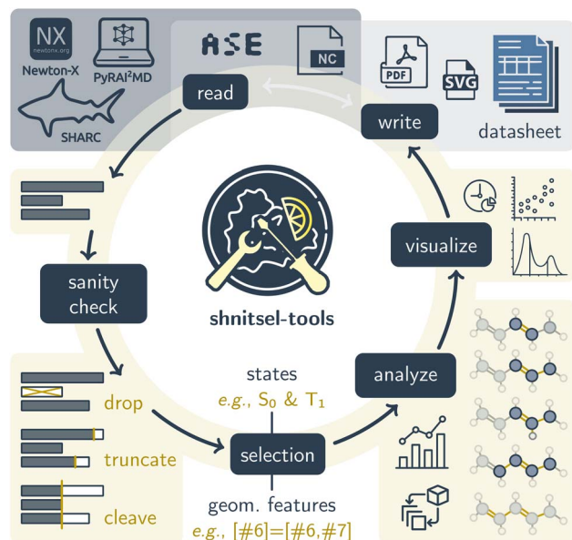
Fig. 1 Schematic overview of the shnitse1-tools ( st ) data lifecycle and analysis workflow. st reads surface-hopping (SH) trajectory data produced by various simulation engines (such as SHARC, PyRAI 2 MD, and Newton-X) via a unified parsing layer, which standardizes their diverse outputs into a hierarchical data model enriched with metadata. A sanity-check stage filters non-physical data based on energetic and geometric criteria. The selection stage then allows restriction of the dataset to specific electronic states or molecular substructures, so that all subsequent operations act only on the chosen subset (or on all states and the full structure if no selection is applied). The analysis stage provides tools for computing geometric descriptors (e.g., bond lengths, angles, dihedrals, pyramidalization) as well as their dimensionality-reduced representations and calculation of statistical observables such as state populations, spectra, and distributions of electronic and geometric properties. The respective results are explored in the visualization stage using time-dependent plots, spectra, scatter plots, and ensemble statistics. Finally, the write stage exports curated datasets in NetCDF format for reproducible storage and sharing, and generates PDF or SVG datashets containing standardized summary plots of the geometry and property space of a certain dataset (e.g., histograms, time plots, absorption spectra) for the selected states and molecular substructures.
