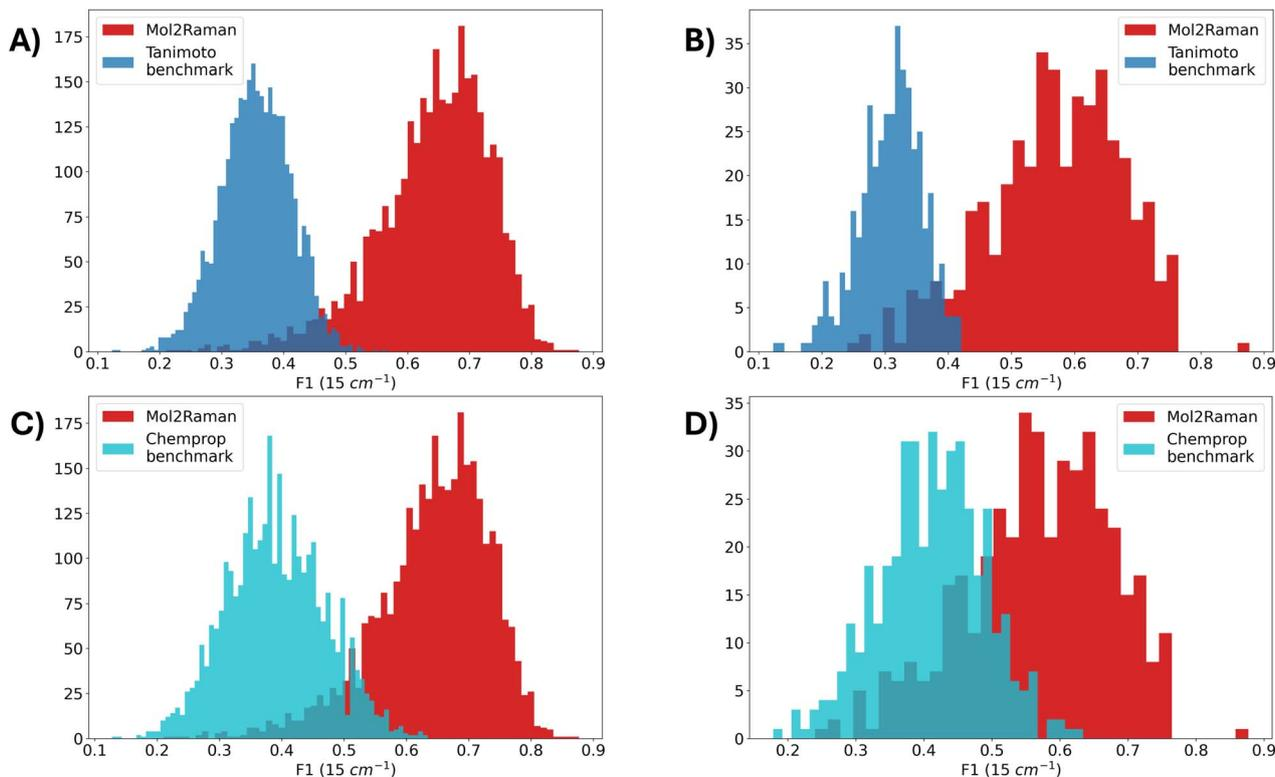
Fig. 6 Comparisons of the distribution of  $F_1$  scores ( $15\text{ cm}^{-1}$  tolerance) for Mol2Raman against benchmark models. (A) and (C) show the comparison of Mol2Raman against the Tanimoto similarity and Chemprop benchmark models on the full test set, while (B) and (D) show the same comparisons on the low-similarity subset of the test dataset (Tanimoto similarity  $<0.6$ ).
