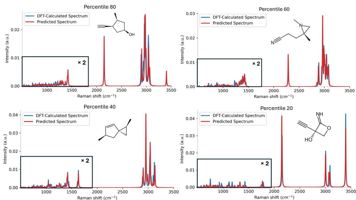
Fig. 4 Comparison of DFT-calculated and Mol2Raman-predicted Raman spectra for different  $F_1$  score percentiles at different percentiles (15  $\text{cm}^{-1}$  tolerance). Raman modes in the fingerprint region are multiplied by a factor of 2 to provide a better comparison.
