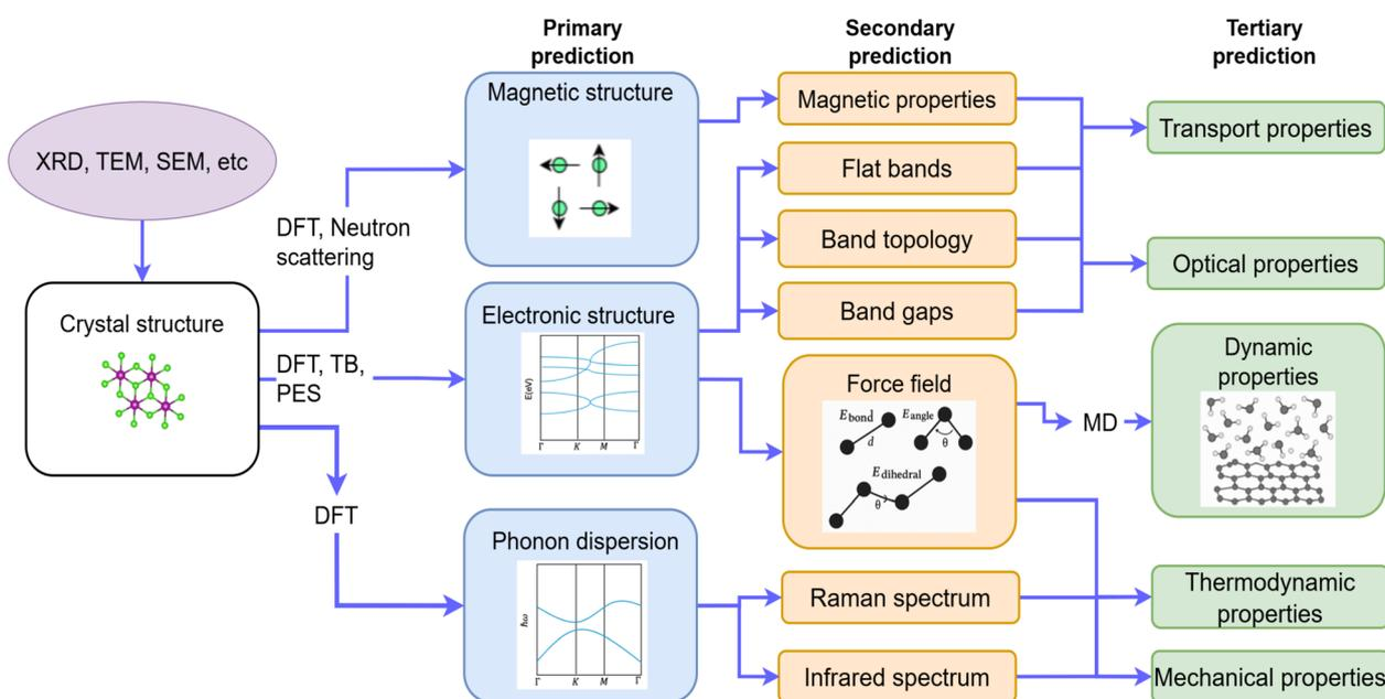
Fig. 3 Forward design pathways for 2D material crystal structures to properties. Crystal structures are validated using experimental techniques like XRD, TEM etc. First principles simulations like DFT calculates electronic, phononic, and magnetic structure which in turn yields end properties like optical, transport, mechanical and dynamic properties.
