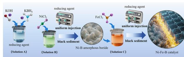
Fig. 1 Synthesis procedure of Ni-Fe-B catalyst.
