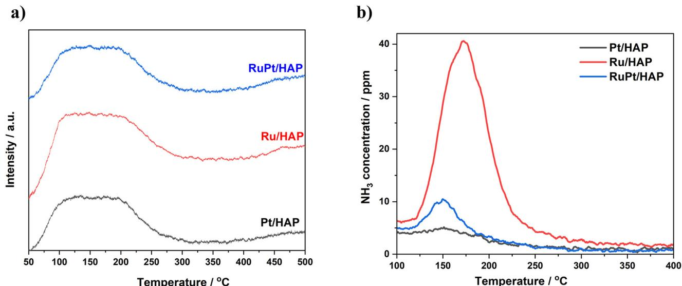
**Fig. 10** Temperature programmed desorption profiles a) CO<sub>2</sub> and b) NH<sub>3</sub> of monometallic and bimetallic nanoparticles supported on HAP.
