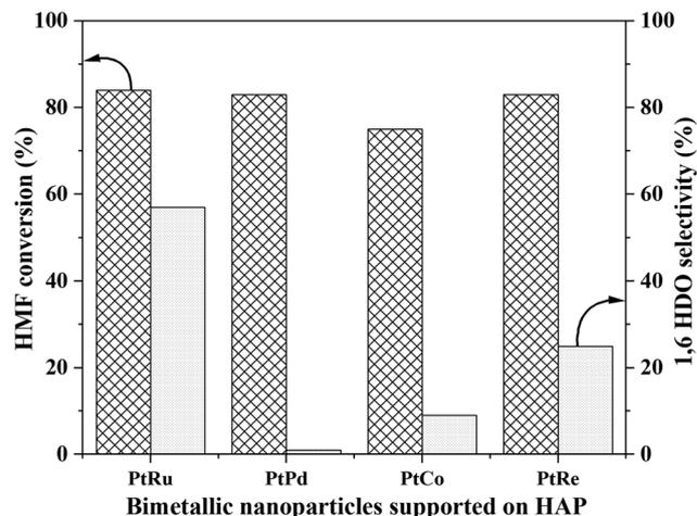
**Fig. 2** Comparison of the catalytic activities of different bimetallic nanoparticles (5wt%) supported on HAP for the ring opening hydrogenolysis of HMF to 1,6-HDO. Reaction conditions: HMF: 1.59 mmol; HMF/total metal molar ratio: 155; methanol: 20 mL;  $\text{H}_2$ : 2 MPa; temperature: 120 °C; stirring: 1000 rpm; time: 8 h.
