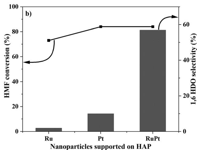
**Fig. 3** Comparison of the catalytic activities of monometallic and bimetallic nanoparticles (5%) supported on HAP for the ring opening hydrogenolysis of HMF to 1,6-HDO. Reaction conditions: HMF: 1.59 mmol; HMF/metal molar ratio: 155; Methanol: 20 mL;  $\text{H}_2$ : 2 MPa; temperature: 120°C; stirring: 1000 rpm; time: 8 h.
