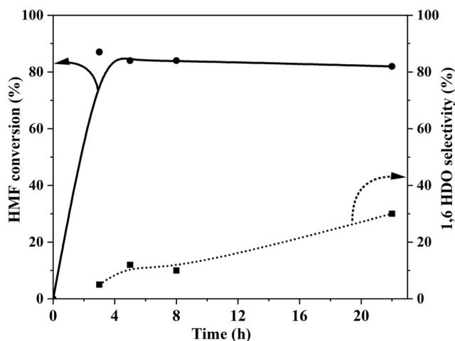
**Fig. 1** Time on line catalytic data for the ring opening hydrogenolysis of HMF to 1,6-HDO over monometallic 5% Pt/HAP. Reaction conditions: HMF: 1.59 mmol; HMF/Pt molar ratio: 155; methanol: 20 mL;  $\text{H}_2$ : 2 MPa; temperature: 120 °C; stirring: 1000 rpm.
