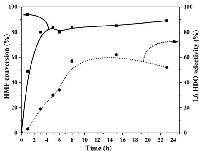
Fig. 4 Time on line data for the ring opening hydrogenolysis of HMF to 1,6-HDO over bimetallic 5% PtRu/HAP. Reaction conditions: HMF: 1.59 mmol; HMF/Total metal molar ratio: 155; methanol: 20 mL; H<sub>2</sub>: 2 MPa; temperature: 120°C; stirring: 1000 rpm.
