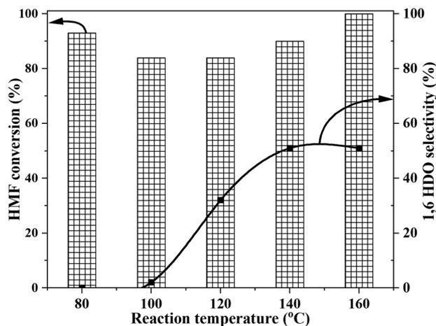
Fig. 7 Effect of reaction temperature during the ring opening hydrogenolysis of HMF over 5% RuPt/HAP. Reaction conditions: HMF: 1.59 mmol; methanol: 20 mL; H<sub>2</sub> pressure: 2MPa; time: 5h; HMF/total metal molar ratio: 155.
