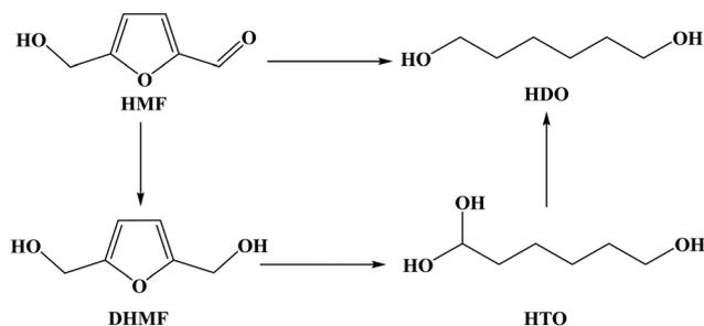
**Scheme 1** Schematic representation of the conversion of HMF to 1,6-hexanediol over supported metal nanoparticles. HMF: 5-hydroxymethylfurfural; DHMF: 2,5-dihydroxymethylfurfural; HTO: 1,1,6-hexanetriol; and HDO: 1,6-hexanediol. Other intermediate products have been omitted for clarity.
