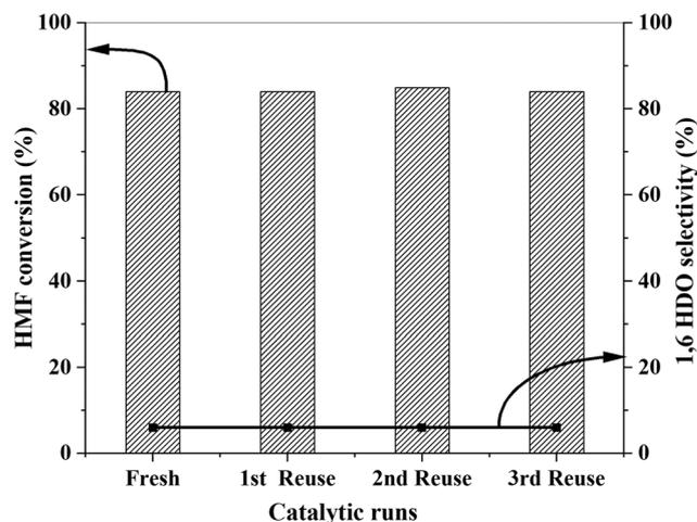
Fig. 5 Reusability of 5% PtRu/HAP catalyst. Reaction conditions: HMF: 1.59 mmol; HMF/Pt molar ratio: 155; methanol: 20 mL; H<sub>2</sub>: 2 MPa; temperature: 120°C; stirring: 1000 rpm; time: 2h.
