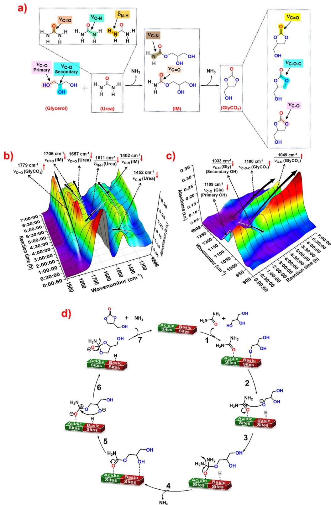
Fig. 7 a) Reaction pathway and functional group assignment in the synthesis of GlyCO<sub>3</sub>. b) and c) 3-Dimensional spectra of the glycerolysis of urea monitored over ALN1Zn2 (catalyst loading = 10%, 150 °C, 7 h, G : U = 1 : 1, N<sub>2</sub> flow, 700 rpm). d) Plausible mechanism of GlyCO<sub>3</sub> synthesis from urea and glycerol on the ALN1Zn2 catalyst surface.
