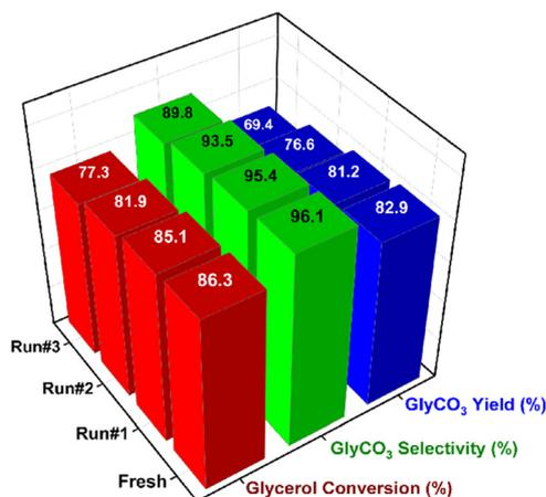
Fig. 6 Recycle run of ALN1Zn2 at 150 °C in 7 h, catalyst loading = 10 %, G : U = 1 : 1, N<sub>2</sub> flow, 700 rpm.
