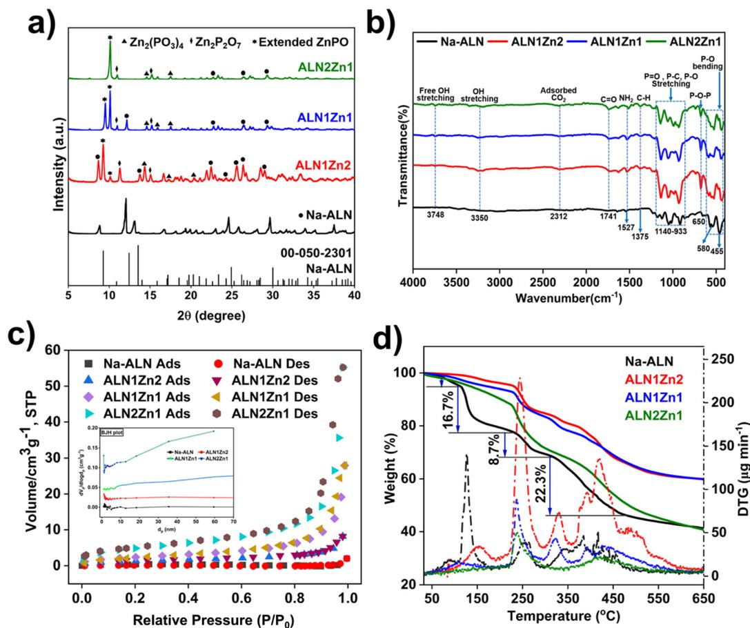
Fig. 1 a) PXRD patterns, b) FT-IR spectra, c)  $N_2$  physisorption plots and BJH pore size distribution plots (inset), and d) TGA spectra of Na-ALN and ossified zinc alendronate catalysts.
