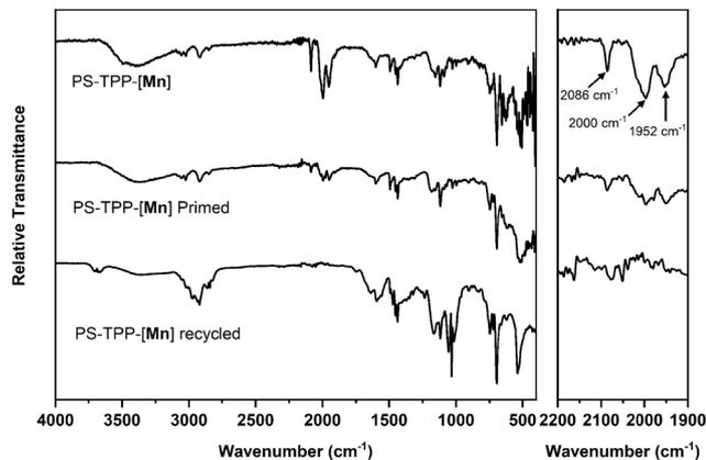
Fig. 2 FTIR analysis comparison of unused (top), primed (centre) and recycled (bottom) catalyst. The right-hand panel shows an expansion of the region between 2200 and 1900  $\text{cm}^{-1}$ .
