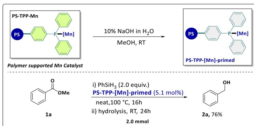
Scheme 3 Reduction using ‘primed’ heterogeneous Mn catalyst.
