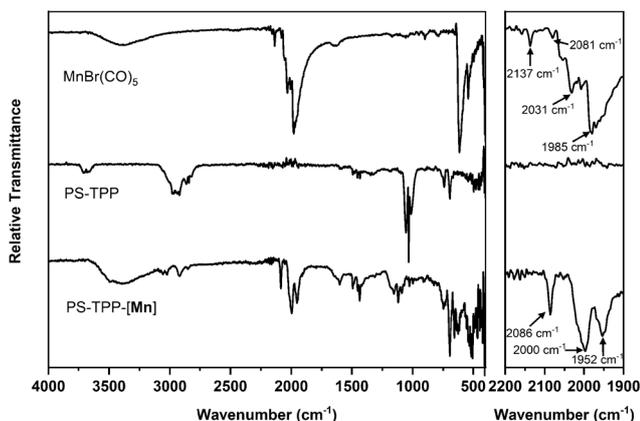
Fig. 1 ATR-FTIR analysis for MnBr(CO)<sub>5</sub> (top), PS-TTP (centre) and PS-TTP-[Mn] (bottom). The right-hand panel shows an expansion of the region between 2200 and 1900 cm<sup>-1</sup>.
