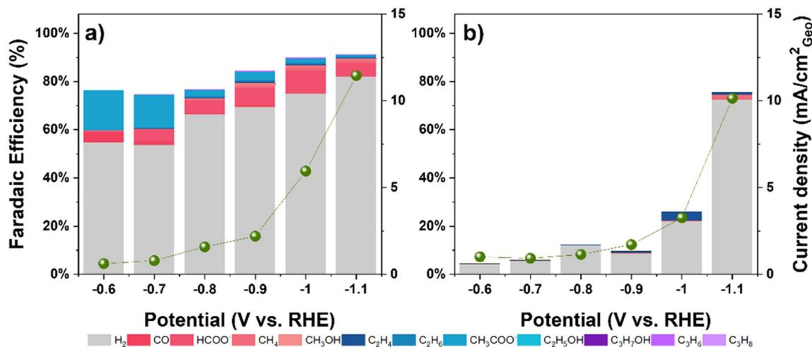
Fig. 7 Faradaic efficiency of products on NiCu-C catalyst during a) CO<sub>2</sub> reduction and b) CO reduction in 0.1 M KHCO<sub>3</sub> + 0.05 M KOAc solution.
