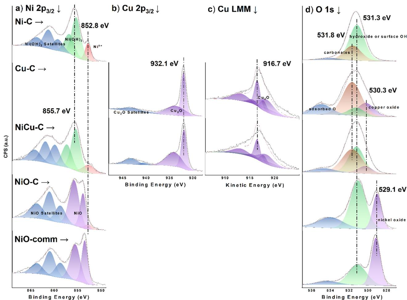
Fig. 3 XPS spectra of (a) Ni 2p<sub>3/2</sub>, (b) Cu 2p<sub>3/2</sub>, (c) Cu LMM, and (d) O 1s regions for Ni-C, Cu-C, NiCu-C, NiO-C, and NiO-comm samples after CO<sub>2</sub>RR. Blank spaces in (b) and (c) indicate the absence of a detectable Cu signal.
