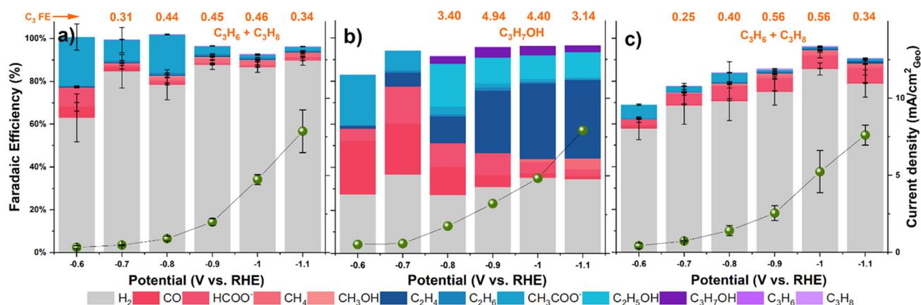
Fig. 4 Faradaic efficiency of products on a) Ni-C, b) Cu-C and c) NiCu-C catalysts during CO<sub>2</sub> reduction in 0.1 M KHCO<sub>3</sub> solution. C<sub>3</sub> products FEs are labelled for easy comparison. Error bars for (a) and (c) represent the standard deviation from independent replicate measurements; values in panel (b) are from a single benchmark experiment.
