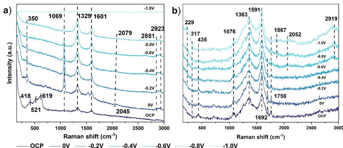
Fig. 8 *In situ* Raman spectra of a) Cu-C and b) Ni-C in CO<sub>2</sub> saturated 0.1 M KHCO<sub>3</sub> from OCP to -1.0 V vs. RHE.
