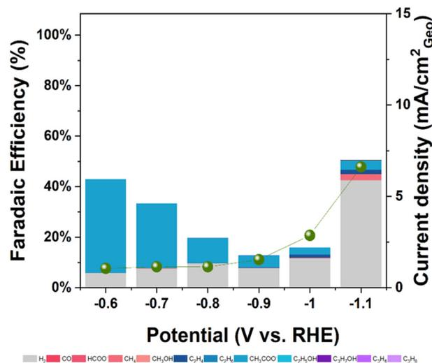
Fig. 6 Faradaic efficiency of products on NiCu-C catalyst during CO reduction in 0.1 M KHCO<sub>3</sub> solution.
