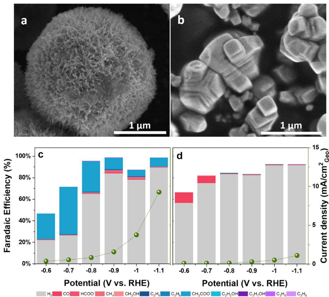
Fig. 5 a and b) SEM images; c and d) faradaic efficiency of products on NiO-C (left) and commercial NiO (right) catalysts during CO<sub>2</sub> reduction in 0.1 M KHCO<sub>3</sub> solution.
