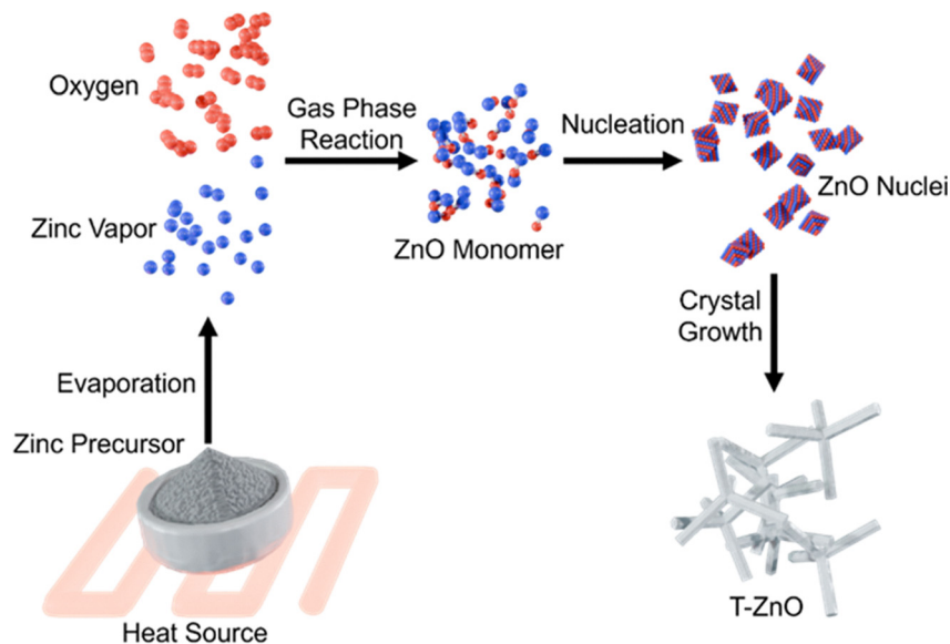
Fig. 7 Schematic overview of the thermal evaporation synthesis route. A heat source vaporizes metallic zinc precursors, which undergo a gas-phase reaction with oxygen to generate ZnO monomers. These monomers aggregate into foundational nuclei and subsequently undergo anisotropic crystal growth to yield the final T-ZnO morphology.
